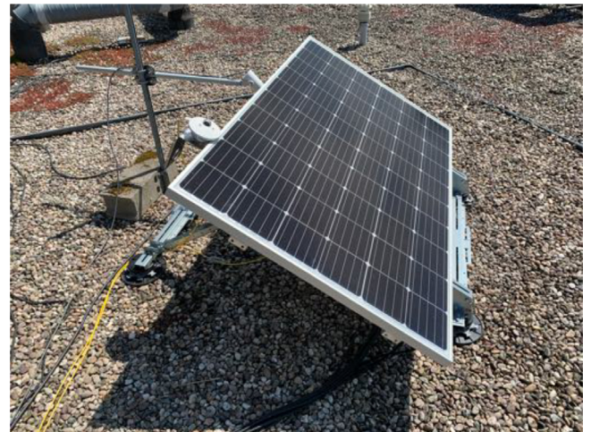
Fig. 9. 310W photovoltaic panel used in the present study in a gravel platform. The pyranometer is in the plane of array of the panel and the pyrometer is pointing under the PV panel. The other sensors are hidden by the PV panel.
