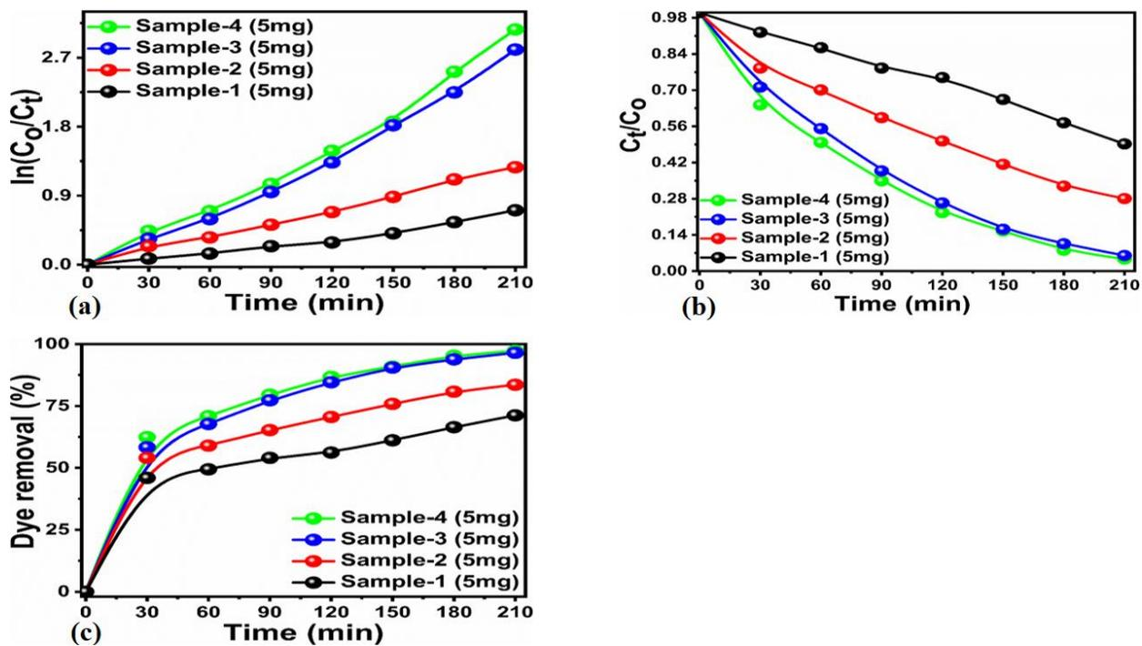
**Figure 7.** Photodegradation kinetics of  $8.22 \times 10^{-5} \text{ M}$  MB solution with catalyst dose of 5 mg of various samples of ZnO such as sample-1, sample-2, sample-3 and sample-4 under the irradiation of natural sunlight, (a) Linear plot of  $\ln(C_t/C_0)$  against corresponding time of 210 min. (b) Linear plot of  $C_t/C_0$ . (c) Degradation efficiency of MB solution using catalyst dose of 5 mg of sample-1, sample-2, sample-3 and sample-4
