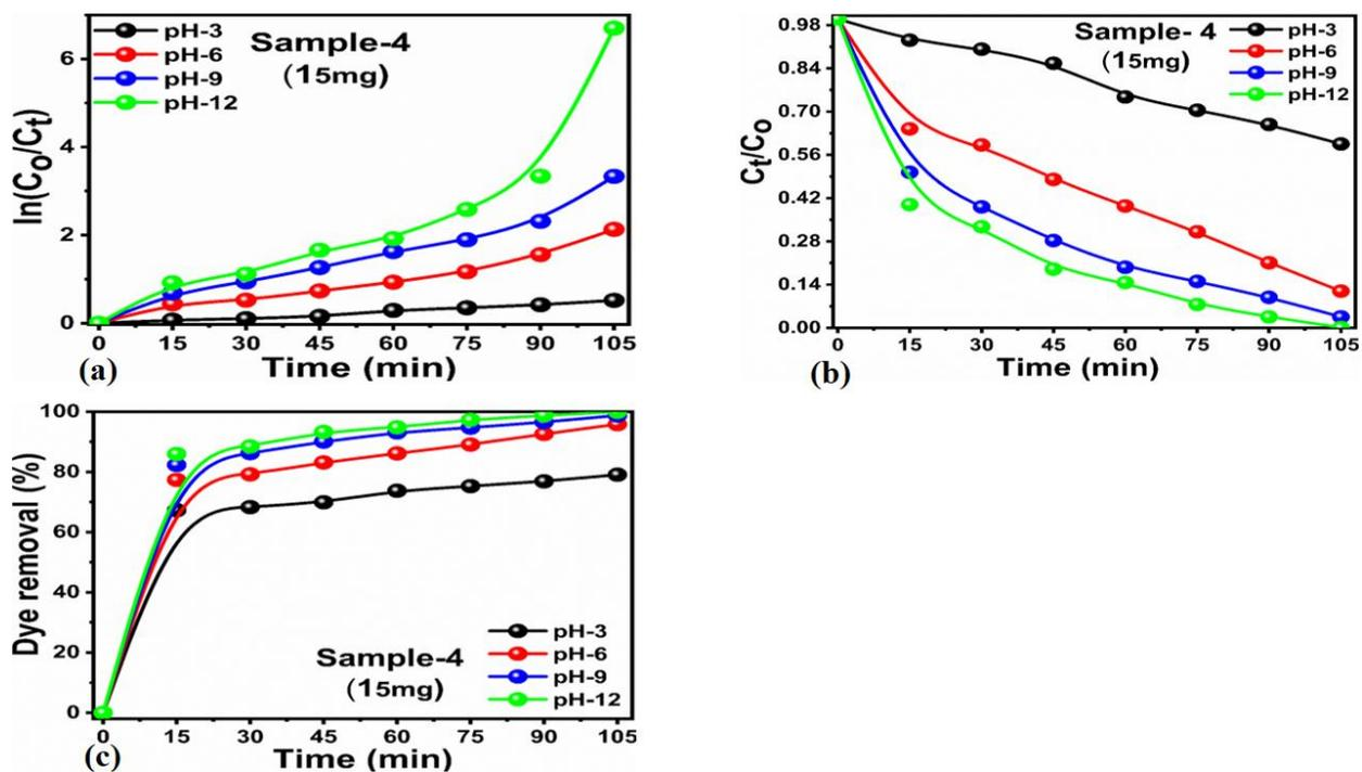
**Figure 14.** Various pH dependent degradation kinetics of  $6.12 \times 10^{-5}$  M MB solution using 15 mg catalyst dose of sample-4 under the irradiation of natural sunlight. (a) Linear plot of  $\ln(C_t/C_0)$  against corresponding time of 105 min. (b) Linear plot of  $C_t/C_0$ . (c) Various pH dependent degradation efficiency of MB solution.
