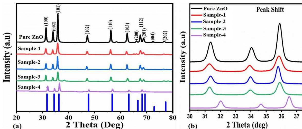
**Figure1.** (a) Powder XRD patterns of pure ZnO and green synthesized ZnO samples prepared with various amount of leafy extract of *S. oleracea* (10 mL, 20 mL, 30 mL and 40 mL) (b) illustrate the shift in (100), (002) and (101) Bragg reflections of as-synthesized samples.
