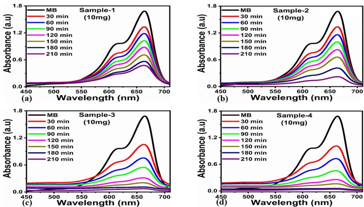
**Figure 8.** (a-d) UV-visible absorption spectra of photodegradation of  $8.22 \times 10^{-5} \text{M}$  MB solution using catalyst dose of 10 mg of different ZnO samples including sample-1, sample-2, sample-3 and sample-4.
