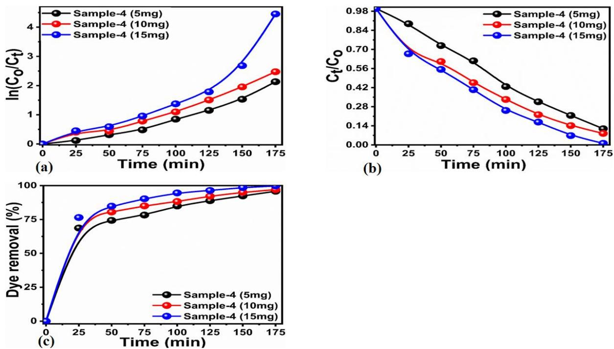
**Figure 12.** Photodegradation kinetics of  $6.12 \times 10^{-5} \text{M}$  MB solution with various catalyst dose of 5 mg, 10 mg and 15 mg of sample-4 under irradiation of natural sunlight (a) Linear plot of  $\ln(C_t/C_0)$  against corresponding time of 175 min. (b) Linear plot of  $C_t/C_0$ . (c) Various pH dependent degradation efficiency of MB solution.
