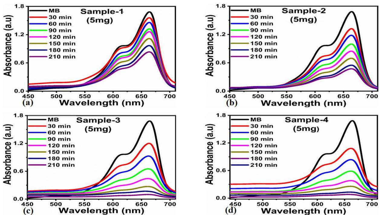
**Figure 6.** (a-d) UV-visible absorption spectra of photodegradation of  $8.22 \times 10^{-5} \text{ M}$  MB solution using catalyst dose of 5 mg of sample-1, sample-2, sample-3 and sample-4 under the irradiation of natural sunlight
