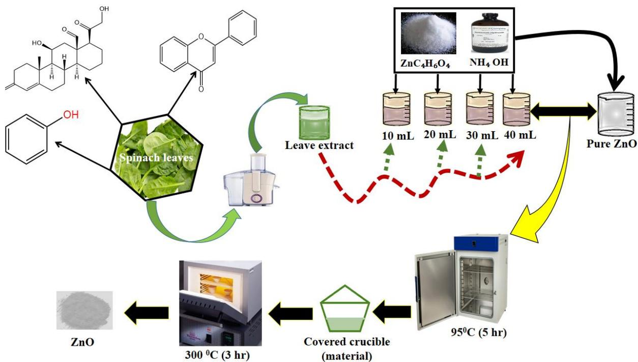
**Scheme 1.** Material synthesis illustration of as-synthesized ZnO samples treated with different amount of leafy extract of *S. oleracea*.
