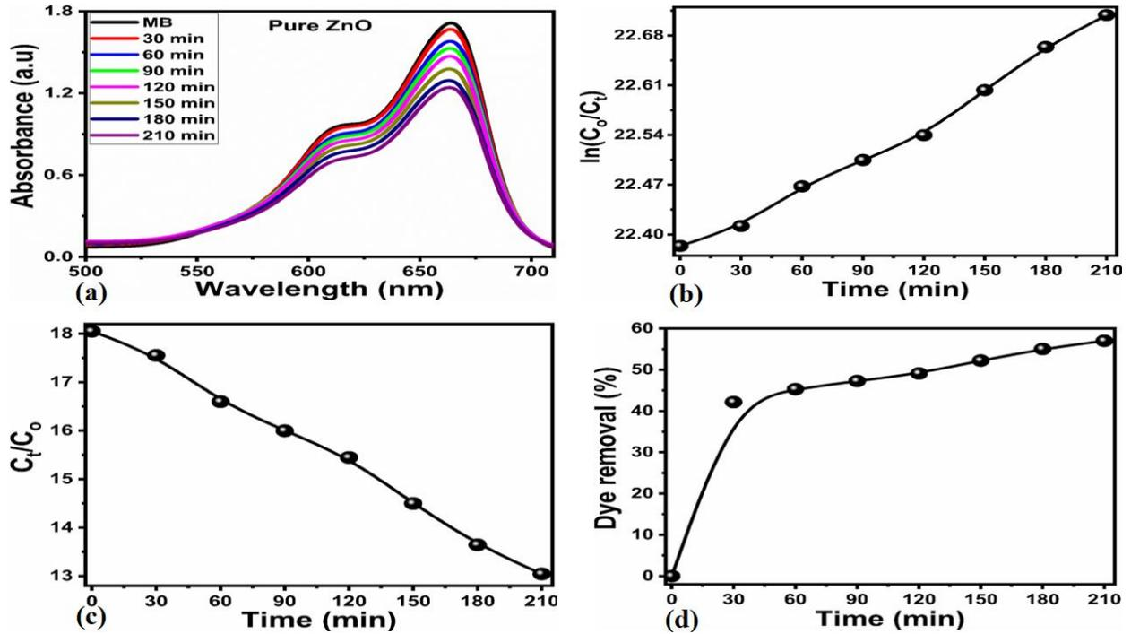
**Figure 5.** (a) UV-visible absorption spectra of  $8.22 \times 10^{-5}$  M) MB solution using photocatalyst dose of 15 mg of pure ZnO for the time interval of 210 min under the irradiation of natural sunlight, (b) Linear plot of  $\ln(C_t/C_0)$  against corresponding time of 210 min. (c) Linear plot of  $C_t/C_0$ . (d) Degradation efficiency of MB solution
