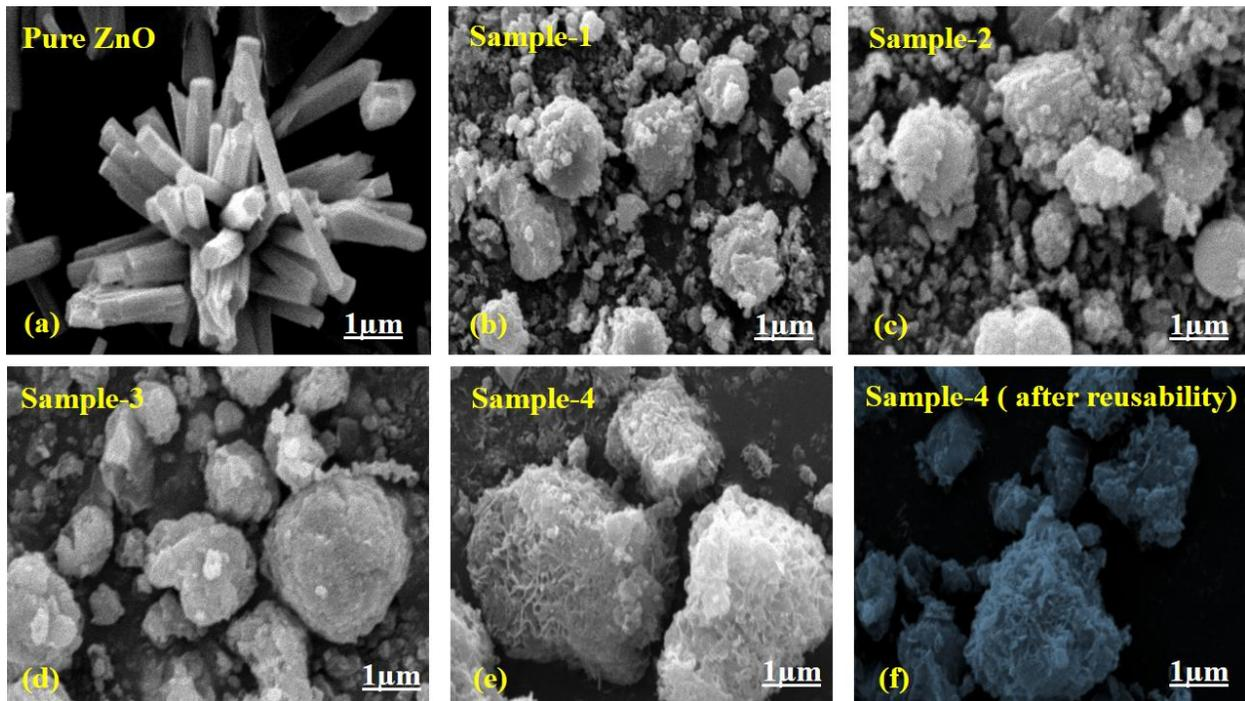
**Figure 2.** SEM images of (a) pure ZnO (b-e) green synthesized ZnO samples treated with different amounts of leafy extract of *S. oleracea* (10 mL, 20 mL, 30 mL and 40 mL) and (f) SEM image after reusability test.
