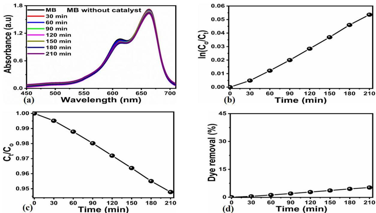
**Figure 4.** (a) UV-visible absorbance spectra measured in  $8.22 \times 10^{-5}$  M MB solution in the absence of catalyst with the irradiation of natural sunlight for the time interval of 210 min, (b) Linear plot of
