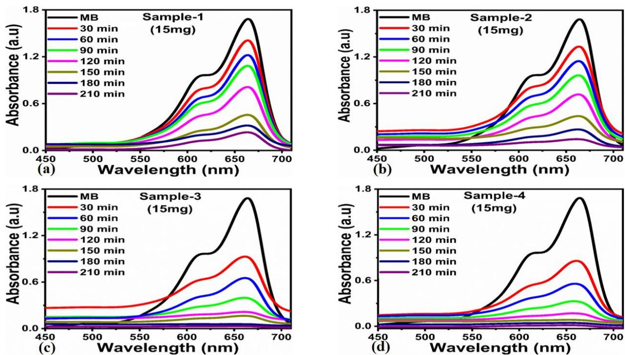
**Figure 9.** (a-d) UV-visible absorption spectra of photodegradation of  $2.2 \times 10^{-5}$  M MB using catalyst dose of 15 mg of various ZnO samples such as sample-1, sample-2, sample-3, and sample-4
