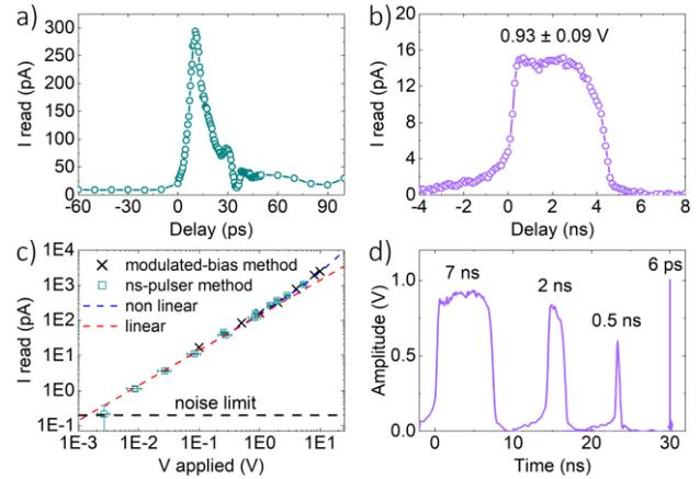
**Fig. 2.** a) A typical picosecond current pulse and b) 4 ns current pulse sampled by detector 1. c) The measured current as a function of the applied voltage to the detector, either statically (modulated bias method) or as pulses (nanosecond-pulsar method). Both methods give the same linear response. d) A few examples of pulses of variable amplitude detected by detector 1 ranging from 7 ns to 6 ps.
