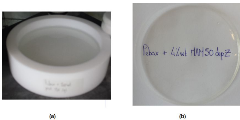
Figure S14. (a) Evaporation of butanol during membrane casting on a PTFE mold, and (b) example of a prepared membrane containing 4.0 wt% of the deprotected trimer ( 7c' ) pseudopeptide as additive in Pebax ® 1074 polymer before gases separation test.
