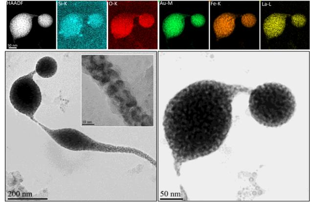
**Fig. 4.** Top: HAADF image and EDX elemental maps of elongated particles connected by 1D-assembly of particles of  $\sim 6\text{-}9$  nm. Bottom left: larger view of the whole object. Insert: High-resolution image of 1D connection. Bottom right: TEM image showing the porous structure of the assembled particles.
