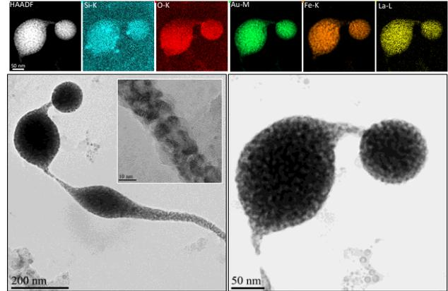
**Fig. 4.** Top: HAADF image and EDX elemental maps of elongated particles connected by 1D-assembly of particles of ~6-9 nm. Bottom left: larger view of the whole object. Insert: High-resolution image of 1D connection. Bottom right: TEM image showing the porous structure of the assembled particles.
