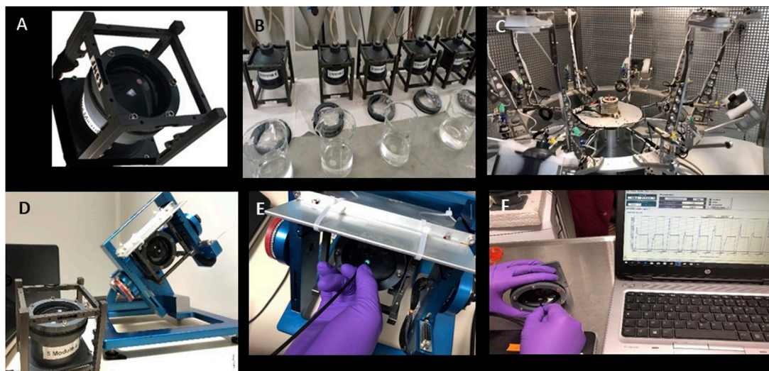
FIGURE 2 (A), (B) Experimental tank (230 mL) inside a CubeSat (n = 100 eggs) used in this experiment as well as in previous experiments to assess the impact of rocket launch vibrations on aquaculture fish hatching rate (C) Aquatic rotor (from 1 g to 5 g) with experimental tanks in triplicate containing European seabass embryos (n = 100 each) (D) Random positioning machine with a CubeSat containing European seabass embryos (n = 100) exposed for 39 h of simulated microgravity and the control CubeSat (n = 100) (E) Pst3 oxygen sensor and light transmitted by the optical fiber to the sensor spot for oxygen concentration measurement inside of the CubeSat window (F) Oxygen level concentration data transfer to the computer.
