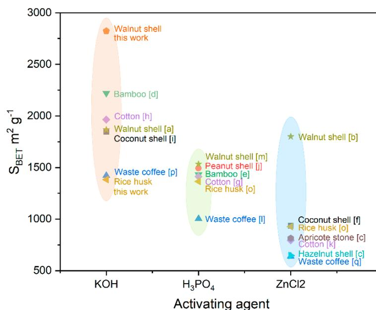
**Figure 1.** A comparison of the  $S_{\text{BET}}$  and activating agents of the reported literature towards chemical activation of different biomass. The corresponding references are shown in Table S1.
