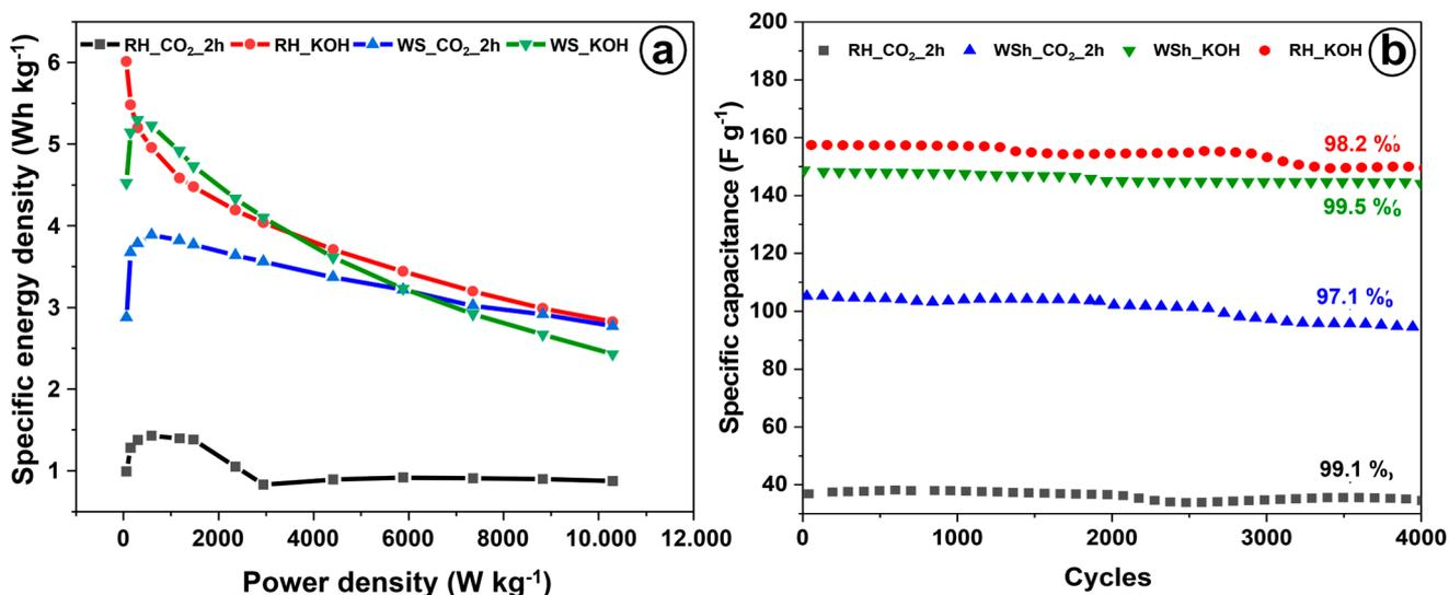
Figure 7. (a) Ragone plot for the rice husk and walnut shell-based electrodes. (b) Cycling GCD test at 2 A g<sup>-1</sup>.
