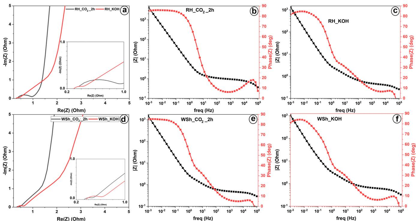
**Figure 8.** Electrochemical performance of KOH-activated and  $\text{CO}_2$ -activated AC derived from rice husk and walnut shell. (a) Nyquist plot recorded in the frequency range of 100 kHz to 0.01 Hz for rice husk-based electrodes and (d) for walnut shell-based electrodes. (b,c) Bode plot for rice husk-based electrodes and (e,f) for walnut shell-based electrodes.
