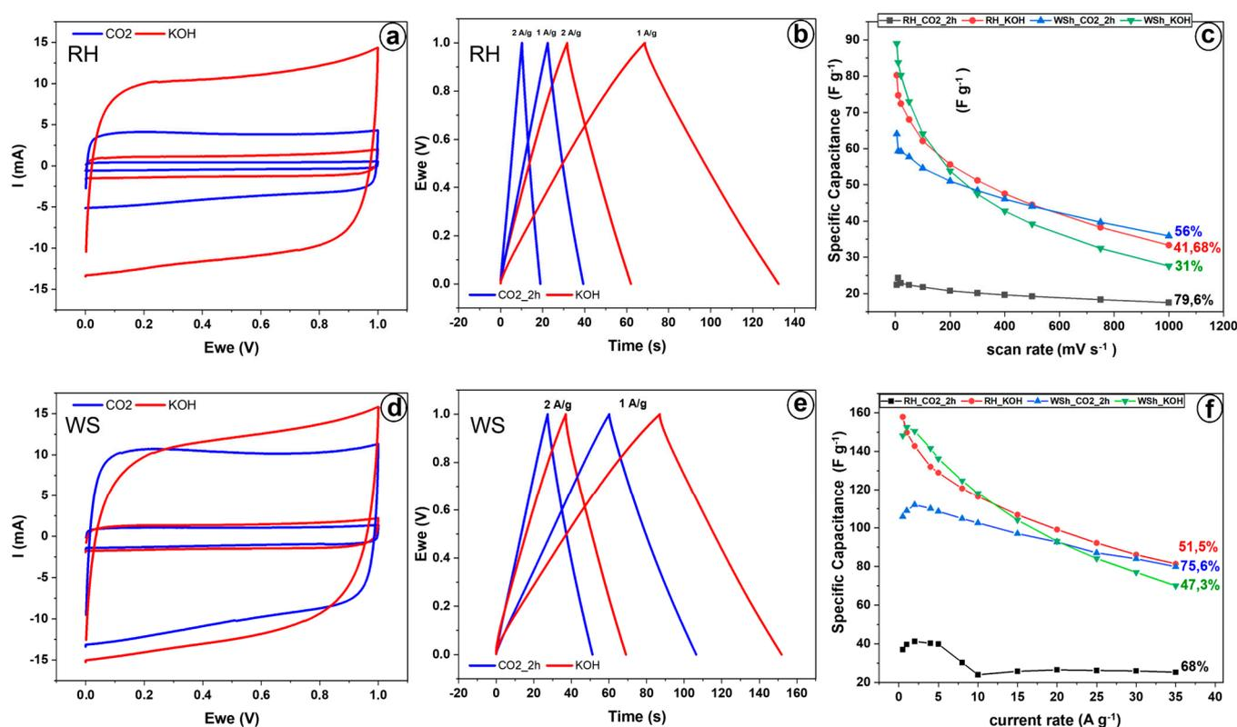
**Figure 6.** Electrochemical performance of KOH-activated and CO<sub>2</sub>-activated AC derived from RH and WS. CV curves at 10 mV s<sup>-1</sup> and 100 mV s<sup>-1</sup> for (a) RH-derived AC and (d) WS-derived AC. GCD curves at 1 A g<sup>-1</sup> and 2 A g<sup>-1</sup> for (b) RH-derived AC and (e) WS-derived AC. Scan rate (c) and current rate (f) capabilities of KOH-activated and CO<sub>2</sub>-activated AC derived from RH and WS.
