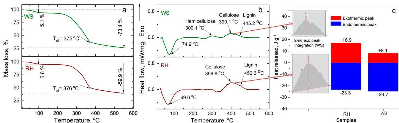
**Figure 5.** Thermal decomposition of WS and RH under nitrogen gas flow ( $100 \text{ cm}^3 \text{ L}^{-1}$ ) at  $5 \text{ K min}^{-1}$  heating rate (a) TG analysis, (b) DSC analysis, and (c) heat release.
