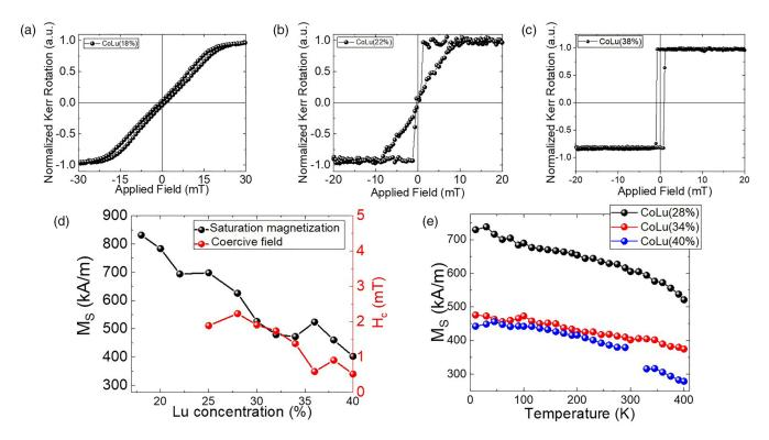
FIG. 1. Typical Kerr rotation hysteresis loops for three different compositions of lutetium: (a) 18%, (b) 22%, and (c) 38%. (d) Variation of the saturation magnetization and coercive field versus the lutetium concentration. (e) Variation of the saturation magnetization versus temperature for  $Co_{1-x}Lu_x$  alloys with concentrations of 28%, 34%, and 40%.
