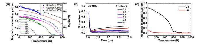
FIG. 5. (a) Magnetic moment versus temperature for  $Co_{1-x}Lu_x$  alloys with various lutetium concentrations, x. Dots indicate experiments; lines indicate simulations. (b) Simulations of the cobalt demagnetization dynamics for the  $Co_{60}Lu_{40}$  alloy as a function of laser power. (c) Simulations of the magnetic moment versus temperature for both cobalt and lutetium subnetworks in case of  $Co_{60}Lu_{40}$ .
