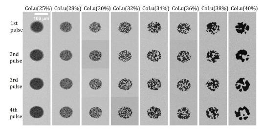
FIG. 2. Domain structure stabilized after 50-fs laser pulses with fluence 6.7 mJ/cm<sup>2</sup>. The images are subtracted by the background, which is saturated by a magnetic field. From left to the right, increasing the lutetium concentration. From top to the bottom, 1 pulse, 2 pulses, 3 pulses, and 4 pulses.
