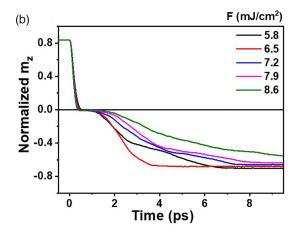
FIG. 6. (a) Demagnetization dynamics for  $J_{\text{Lu-Lu}}$  equal to  $6 \times 10^{-22}$  J when  $\mu_{\text{Lu}} = 4.34 \, \mu_B/\text{atom}$  as a function of fluence. (b) Demagnetization dynamics for  $J_{\text{Lu-Lu}}$  equal to  $6 \times 10^{-21}$  J when  $\mu_{\text{Lu}} = 3.34 \, \mu_B/\text{atom}$  as a function of fluence.
