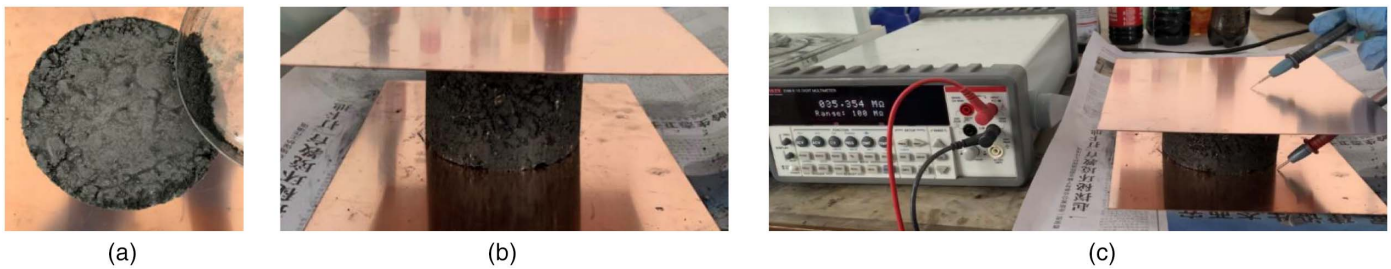
Fig. 5. (a) Graphite layer; (b) placement sequence of the specimen; and (c) position of the probes of the multimeter.
