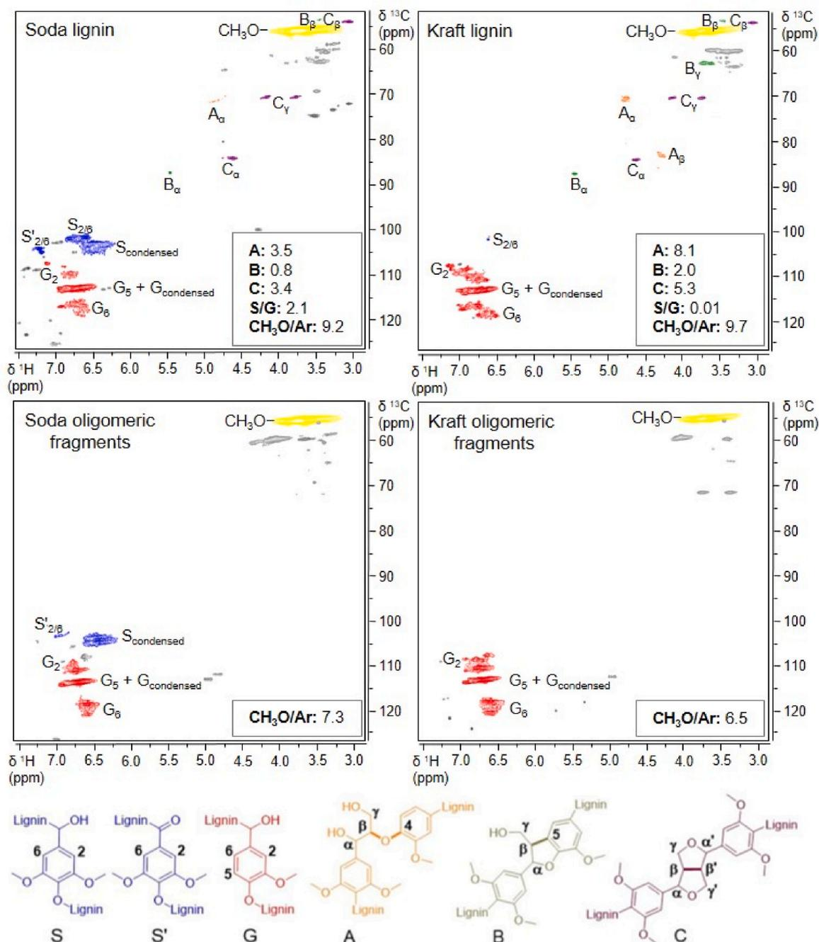
**Fig. 4.** Comparison of the 2D HSQC NMR spectra of Soda and Kraft lignin and its oligomeric fragments following catalytic reaction at 250 °C for 4 h with the Ru/C catalyst ( $H_2$ ). The amounts of the major linkages are calculated per 100C9 units [43].
