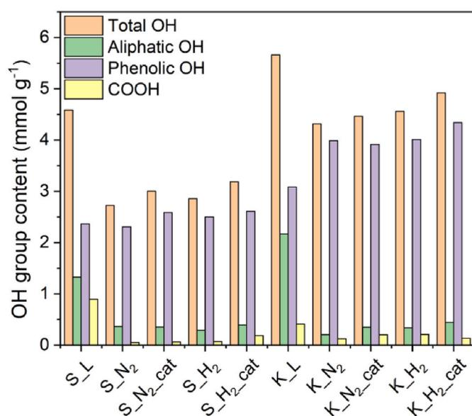
Fig. 6. The change of aliphatic and phenolic OH group content in lignins and oligomeric fragments (S\_L- Soda lignin, S<sub>experimental conditions</sub>- Soda oligomeric fragments after different reaction conditions, K\_L- Kraft lignin, K<sub>experimental conditions</sub>- Kraft oligomeric fragments after different reaction conditions).
