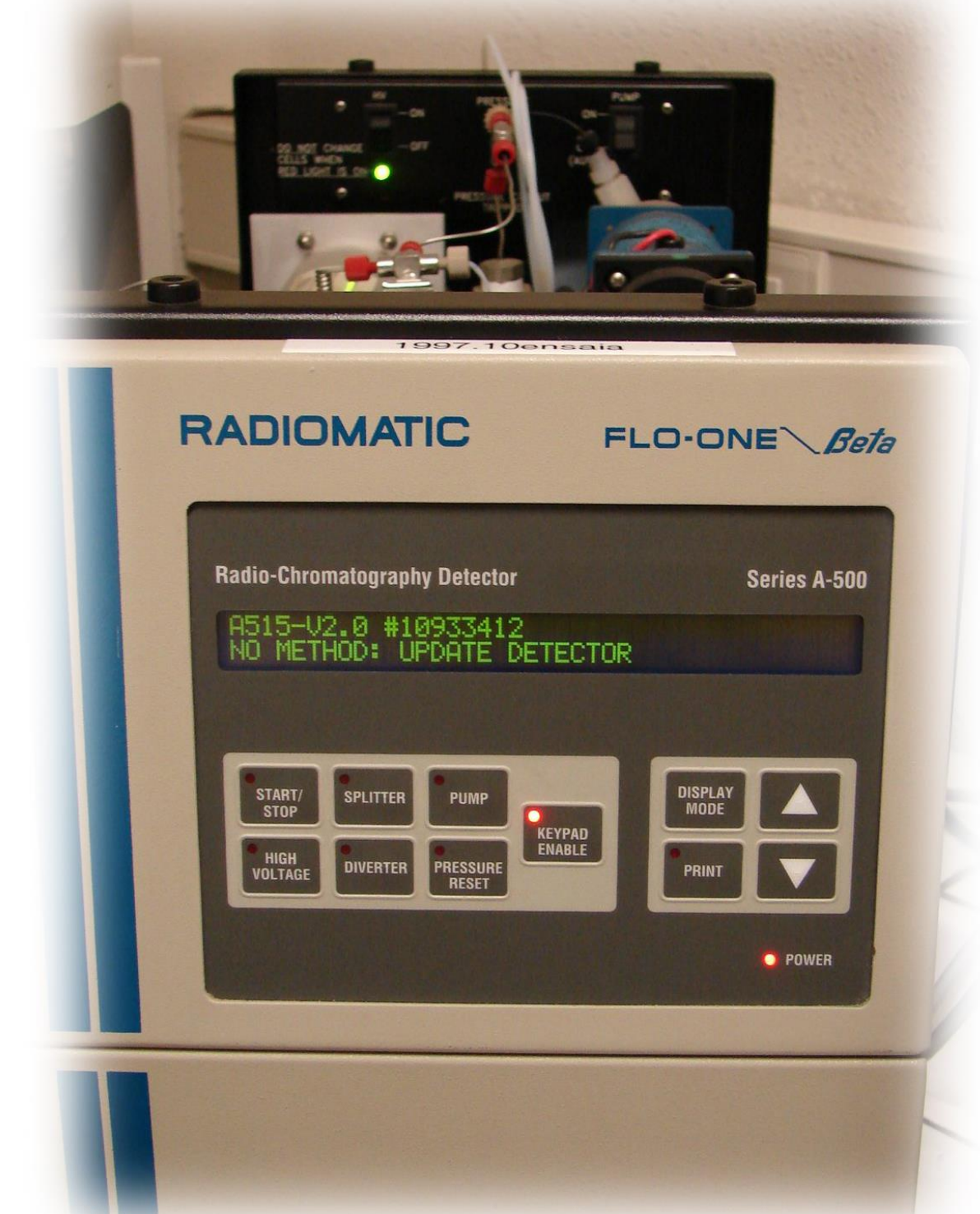
Photo 4. Counting of ^{14}\text{CO}_2 \beta radiations within a 15 ml plastic scintillant cell
