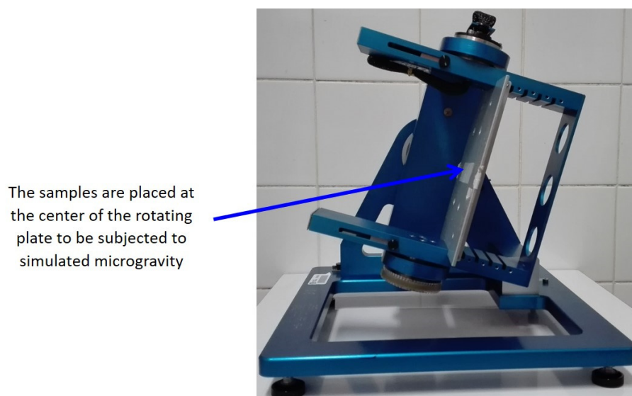
Figure 1. Photograph of the random positioning machine (personal collection). This equipment allows the exposure of biological samples to simulated microgravity. This machine rotates the sample randomly around the Earth's gravity vector resulting in an average net force close to zero, thus simulating microgravity.
