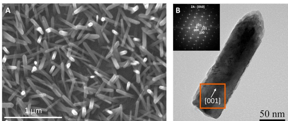
**Fig. 1.** SEM (A) and TEM (B) micrographs (FFT in inset) of Te nanorods electrodeposited in EOPipTFSI:EOPipBr 95:5 (mol%). [TeCl<sub>4</sub>] = 5 mmol·L<sup>-1</sup>. T = 100 °C, Q = 0.1C·cm<sup>-2</sup>.
