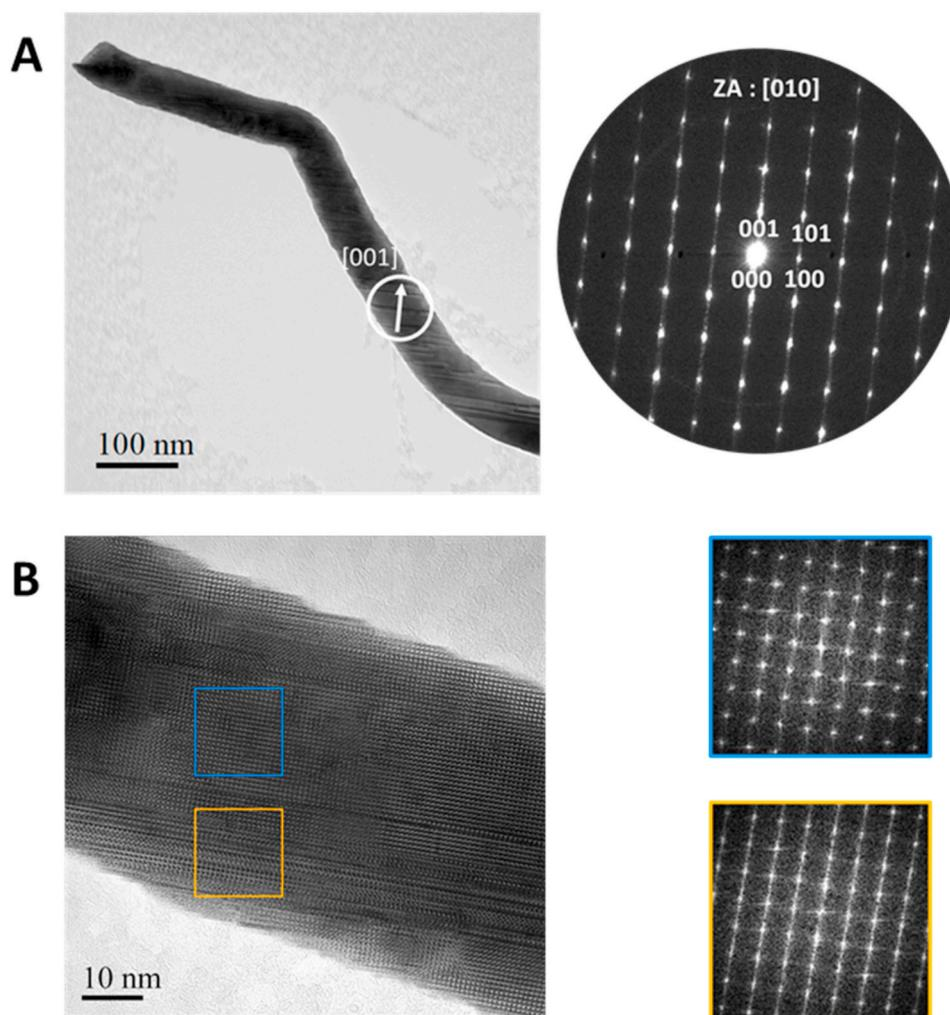
**Fig. 8.** TEM characterizations of copper telluride nanorods after 2 h of reaction in bath B (Cu large excess/ $C_6H_8O_6$  stoichiometry). A) HRTEM and SAED analysis (zone axis [010]) B) HRTEM zoom on growth steps along the nanorods and FFT showing stacking defect (orange) and no defect (blue). (For interpretation of the references to colour in this figure legend, the reader is referred to the Web version of this article.)
