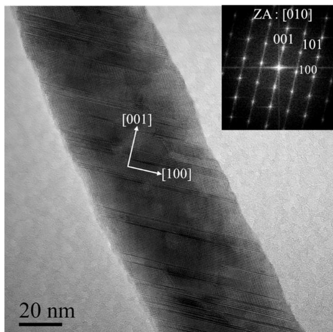
**Fig. 6.** HRTEM micrograph of copper telluride nanorods after 2 h of reaction in bath B (Cu large excess/ $C_6H_8O_6$  stoichiometry) and zooming on the crystallographic structure of  $Cu_7Te_4$  along the [010] zone axis with FFT (SG:  $P\bar{3}m1$  (164) (JCPDS: #04-024-0587).
