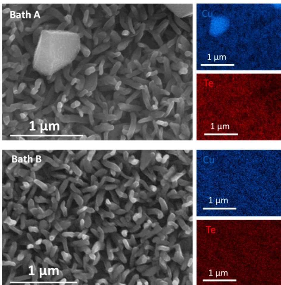
**Fig. 4.** SEM characterizations and corresponding EDX mapping of  $\text{Cu}_7\text{Te}_4$  nanorods film after 2 h immersion in bath A (Cu large excess/ $\text{C}_6\text{H}_8\text{O}_6$  excess) and in bath B (Cu large excess/ $\text{C}_6\text{H}_8\text{O}_6$  stoichiometry).
