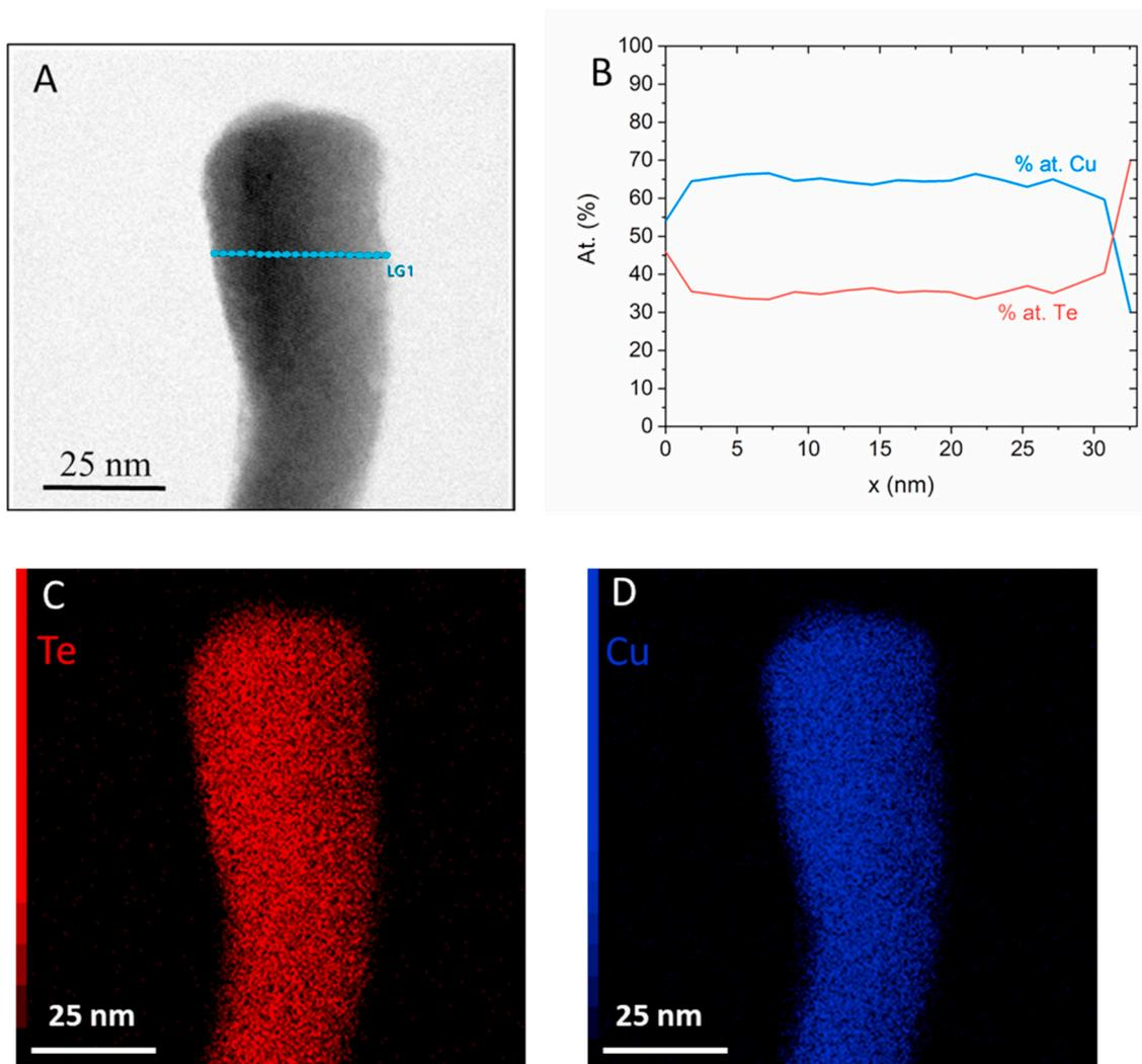
Fig. 5. STEM-EDX characterizations of a Cu<sub>7</sub>Te<sub>4</sub> nanorod after 2 h immersion in bath B (Cu large excess/C<sub>6</sub>H<sub>8</sub>O<sub>6</sub> stoichiometry) (A). EDX line profile (B) and X-ray mapping (C and D).
