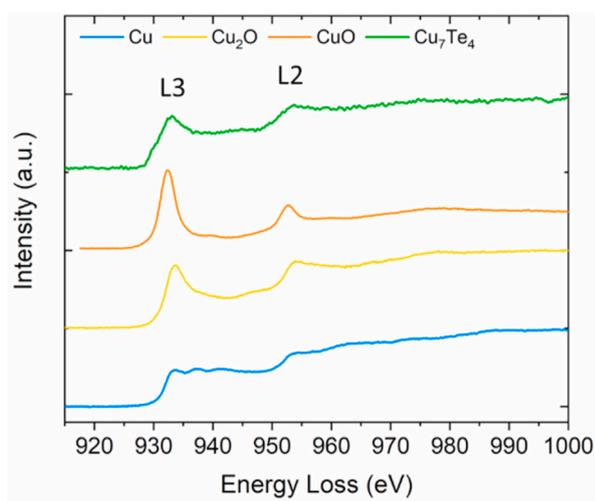
**Fig. 9.** EELS characterization of  $Cu_7Te_4$  nanorods (in green) by comparison with different standards of copper at different oxidation states (Cu in blue,  $Cu_2O$  in yellow and  $CuO$  in orange). (For interpretation of the references to colour in this figure legend, the reader is referred to the Web version of this article.)
