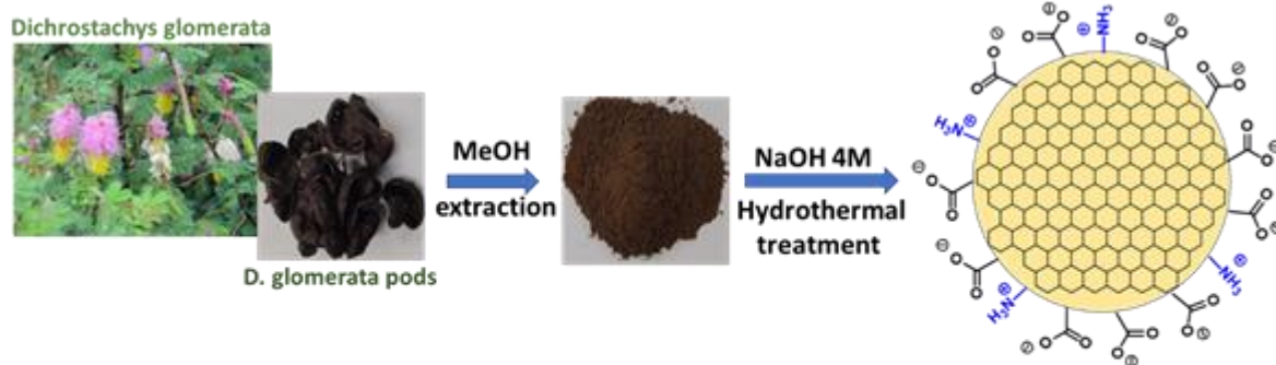
Figure 1. Schematic illustration of CQDs synthesis from D. glomerata pods.
