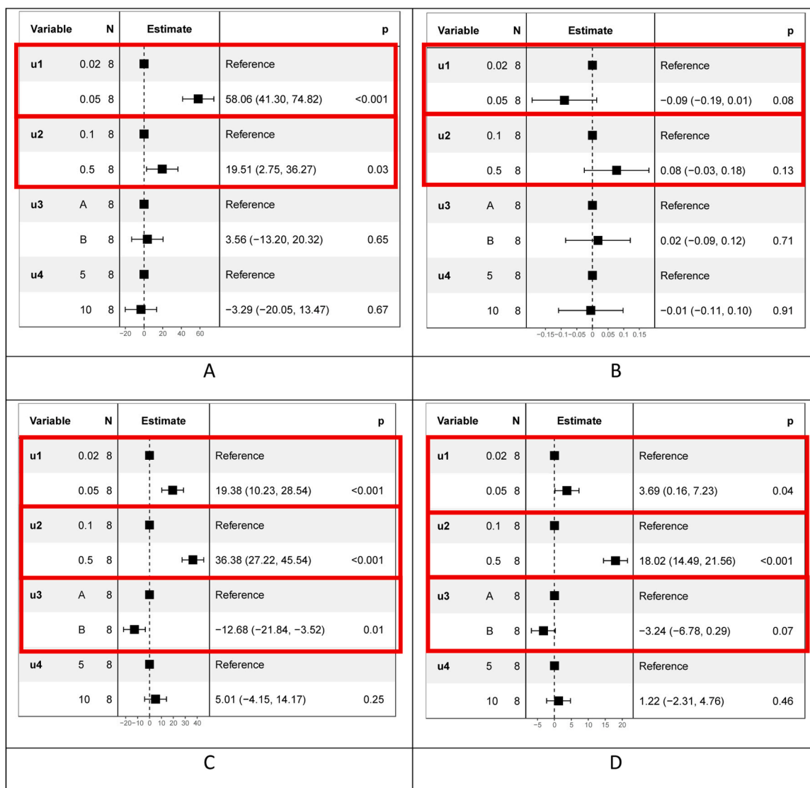
Fig. 4. Forest plots describing statistical results of the screening analysis (Plackett-Burman DoE). A: Effects of the four input factors on the particle size. B: Effects of the four input factors on the polydispersity. C: Effects of the four input factors on the encapsulation efficiency. D: Effects of the four input factors on the drug loading. u1= alginate concentration; u2= drug/polymer ratio; u3= crosslinker addition flow rate; u4= crosslinker volume. The forest plots allow to visualize and summarize the results of the linear regressions. For each factor, the first line corresponds to the reference modality of the factor and the second line to the second modality. Column « N » gives the number of observations for the studied modality. In the Plackett-Burman design, the number of observations is the same for all the modalities. The « estimate » column shows the estimation of the regression coefficient associated to a factor and its confidence interval at 95%. The details are given in the next column: the first value is the estimate of the mean effect on the response value and the values in bracket refers to the lower and upper bounds of the 95% confidence interval. The last value is the p-value of the student t-test on the regression coefficient. The results framed in red correspond to the process parameters estimated as critical.
