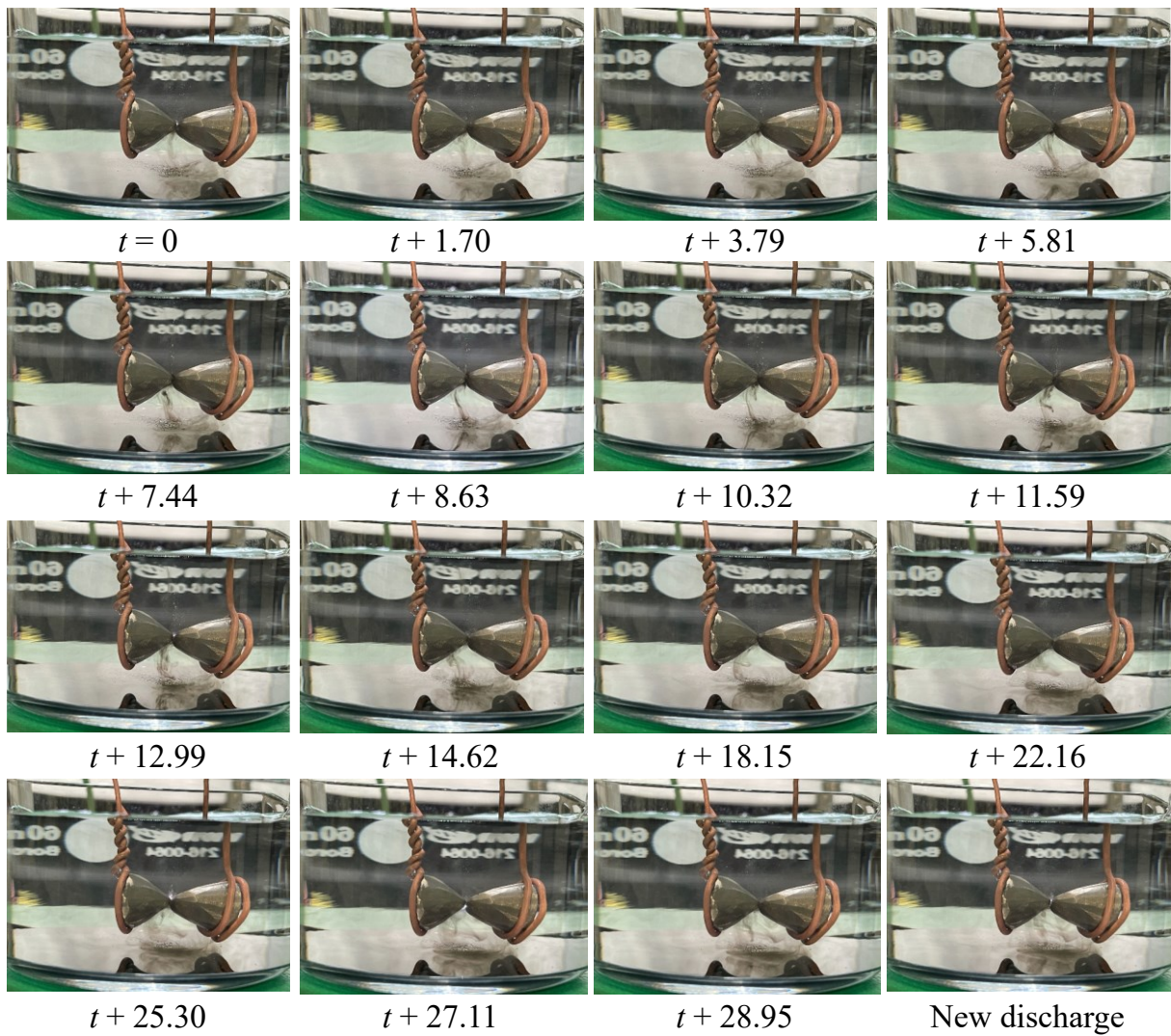
Fig. S11: Set of pictures showing the movement of the generated particles in the liquid between two discharges. The time scale is in second. Particles remain at the bottom of the beaker, settling by gravity.
