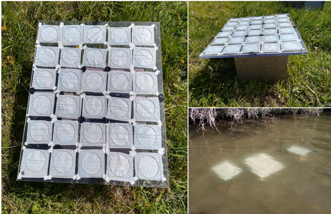
Figure B.1. Masks were sandwiched between two transparent polymethyl methacrylate sheets. The upper sheet was openwork to allow mask colonization by microorganisms during exposure in the river. This experimental device was weighted and horizontally immersed in the Moselle River for 4 weeks.
