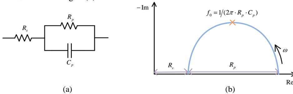
Fig. 2 (a) AC equivalent circuit model connected with a boost converter; (b) An ideal Nyquist curve with several representative parameters
