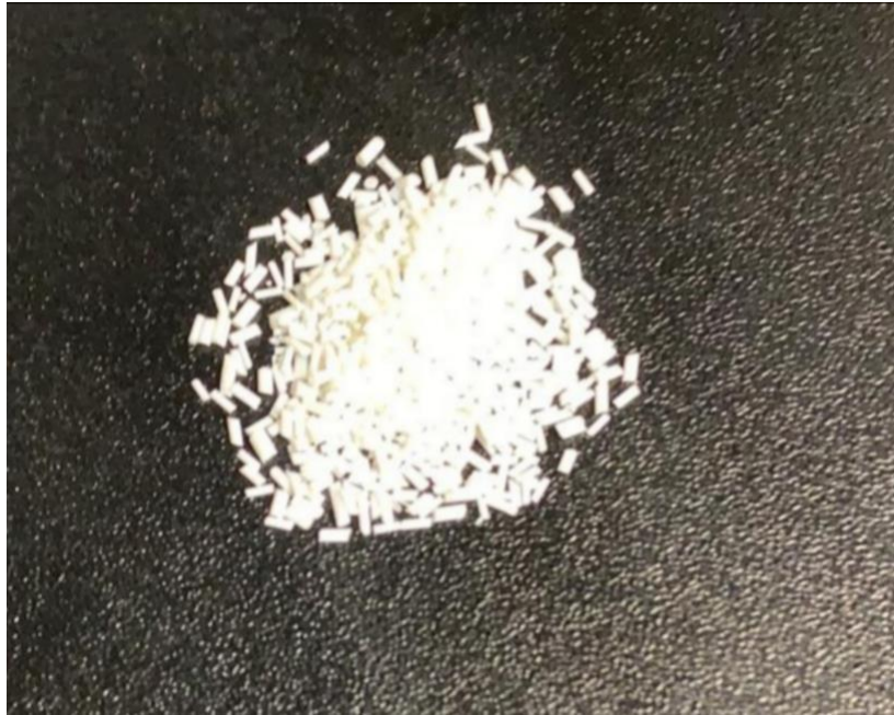
Figure 3. Image of 30% w/w HCQ-loaded Soluplus pellets
