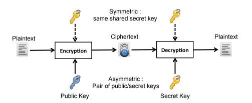
Figure 1: Symmetric Vs. Asymmetric Encryption Schemes.
