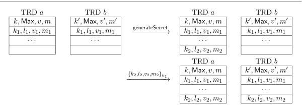
Figure 4.2: A simple execution. A key is created on device a and shared with device b.
