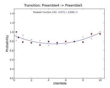
(a) Parabolic function modelling transition PREAMBLE\_4 -> PREAMBLE\_5.
