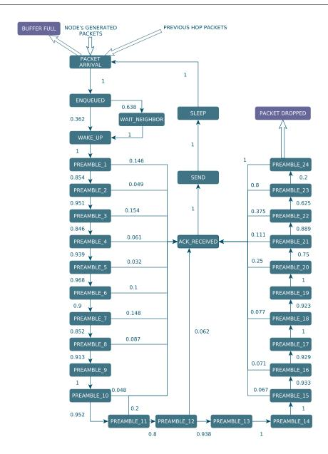
Figure 5.14: Markov chain model for node 166 ( $\lambda = 4$ ).
