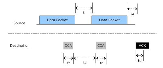
Figure 2.14: ContikiMAC transmission and CCA timing.
