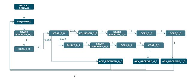
Figure 5.6: Obtained Markov chain of a single device.
