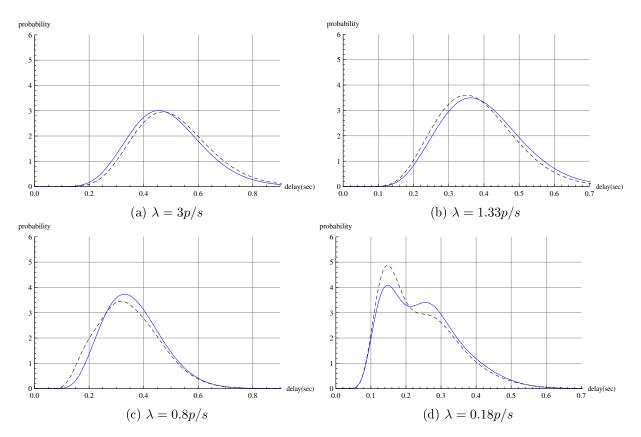
Figure 6.8: Probability density function comparision between non-linear regression approach and empirical results for unknown  $\lambda$  points.
