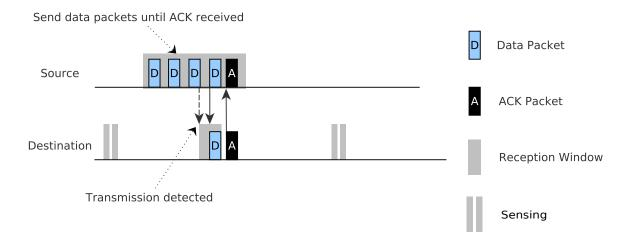
Figure 2.12: ContikiMAC mechanism.
