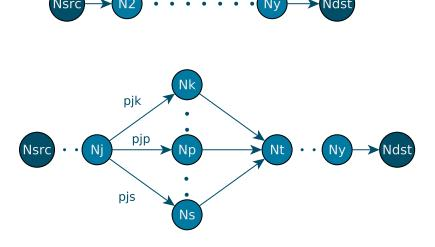
Figure 5.3: Serial (in tandem) and parallel structures.
