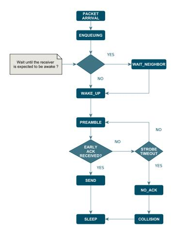
Figure 5.12: State's diagram of X-MAC protocol.
