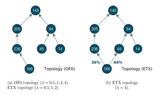
Figure 5.15: Routing graphs for ETX and OF0 objective functions.
