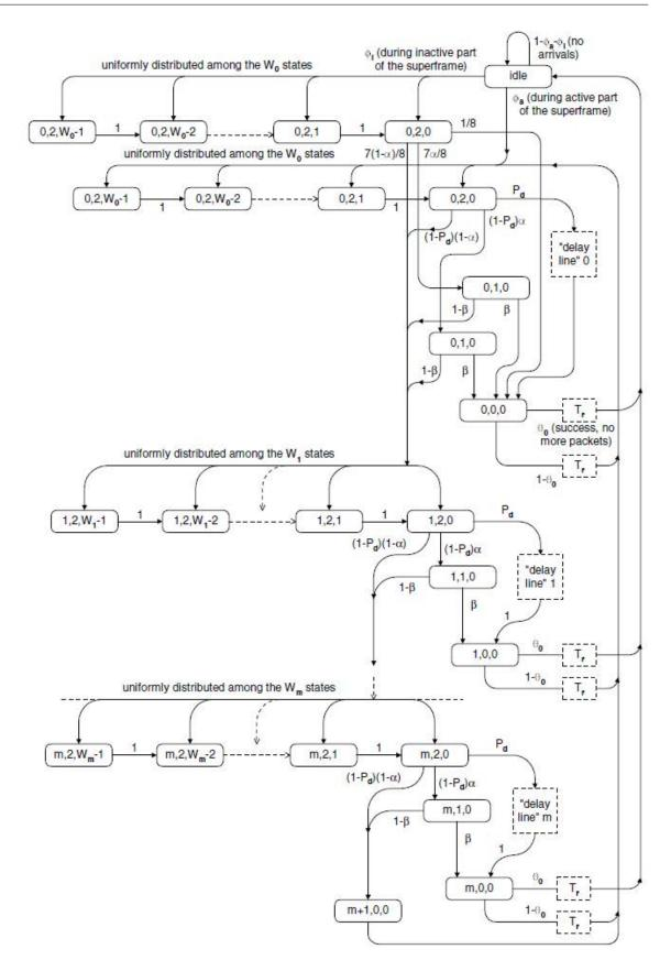
Figure 3.2: Markov chain model of a node executing the slotted CSMA-CA algorithm in a cluster where de superframe has both active and inactive periods [Misic and Misic, 2008]
