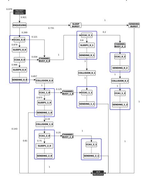
Figure 5.10: Obtained Markov chain for a single device.
