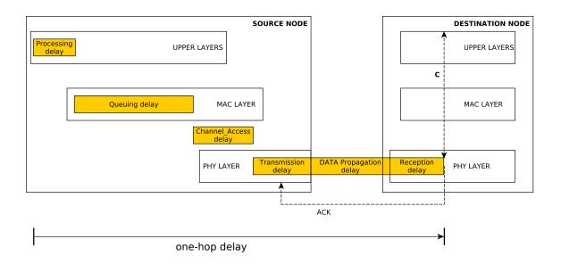
Figure 2.1: One hop delay components.
