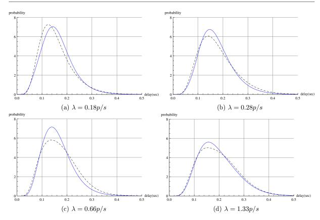
Figure 6.6: Probability density function comparision between non-linear regression approach and empirical results for unknown  $\lambda$  points.
