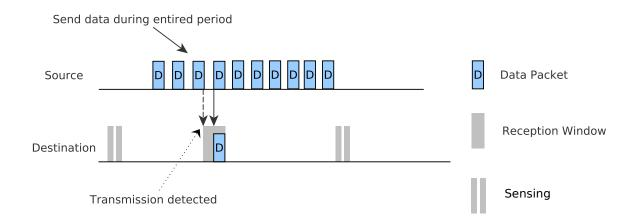
Figure 2.13: ContikiMAC broadcast mechanism.
