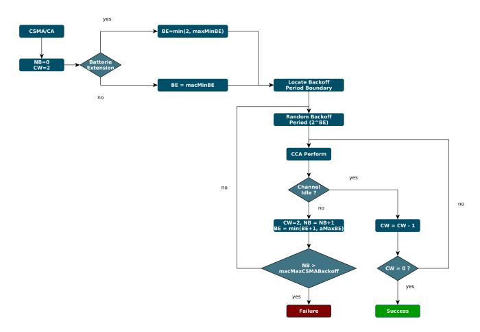
Figure 5.4: IEEE 802.15.4 MAC protocol (slotted version): Flow Diagram.
