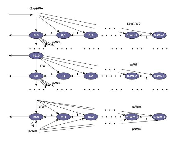
Figure 3.1: Bianchi's Markov chain model for the backoff window size for the standard IEEE 802.11.
