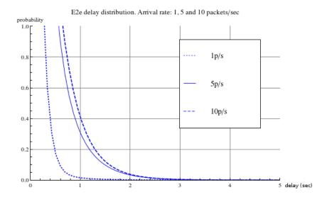
Figure 5.7: Probability distribution function of e2e delay for packet arrival rate  $\lambda = 1, 5, 10 \text{ p/s}$ .
