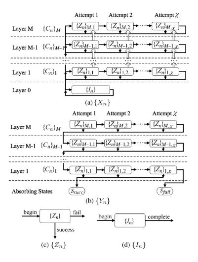
Figure 3.4: Cross-layer Markov chain model to estimate the one-hop delai in one node [Wang et al., 2012].
