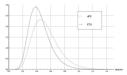
Figure 5.17: Probability density function of the e2e delay from node 166 to the sink (145) for both RPL objective functions (high traffic load scenario).
