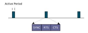
Figure 2.8: S-MAC synchronous periodic wake-up scheme.
