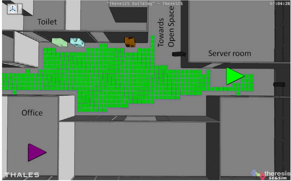
Figure 5.22: 3D representation of the office building environment. The green squares represent areas under sensory coverage. The purple and green triangles are used to model the activities associated with the office room and the server room respectively.
