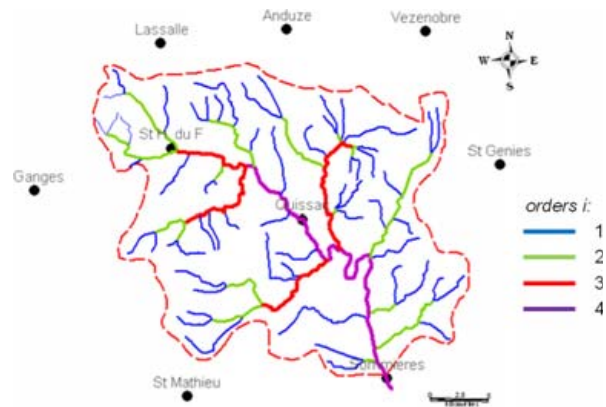
Fig. 4. Example of Strahler classification on a hydrological network (South France) where the Horton–Strahler number is equal to 4.
