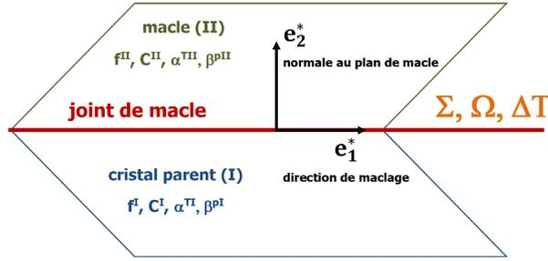
FIGURE 2.4 – Joint de macle plan infini.
