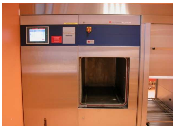
Figure 35 : Autoclave SCHAEERER ECOSTAR®
