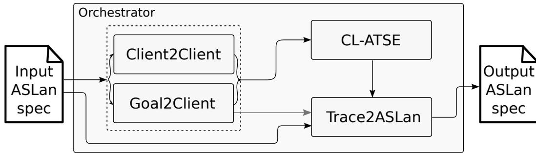
Figure 4.15: Tool architecture
