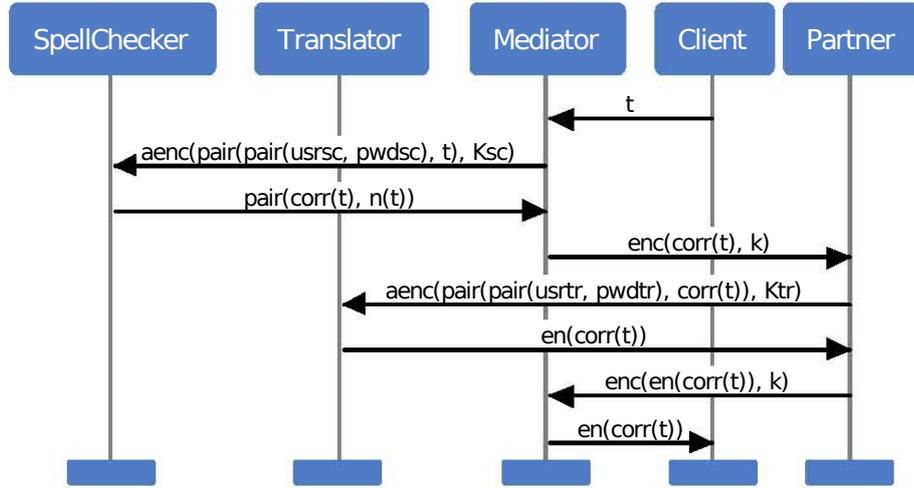
Figure 4.6: Solution for the distributed orchestration problem example
