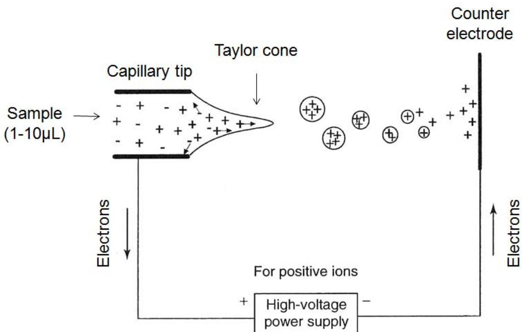
**Figure 12:** Principle scheme of an ESI source (modified from [Hoffman \*et al.\*](#).)
