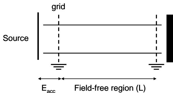
**Figure 22:** Principle of a linear TOF analyzer
