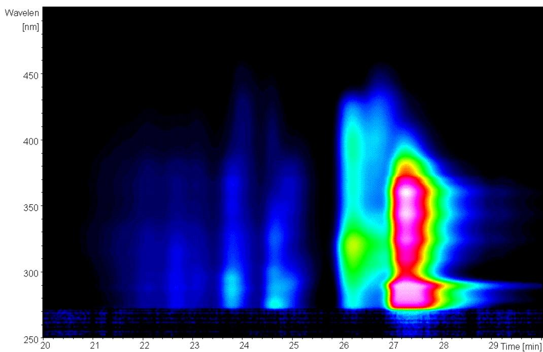
**Figure 6:** UV chromatogram (250-500 nm) for oxy-PAH mixture using a combination of GPC Mixed E + HR columns. Flow rate at 0.3mL/min with a CHCl<sub>3</sub>/C<sub>6</sub>H<sub>6</sub> 90/10 v/v mobile phase.
