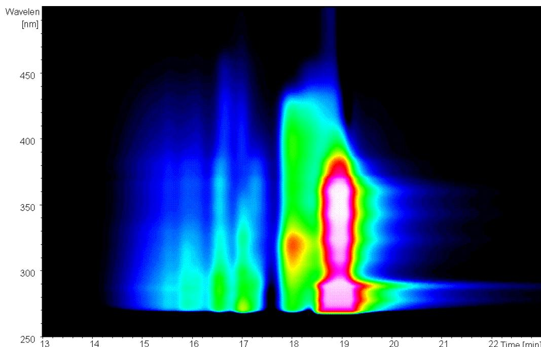
**Figure 4:** UV chromatogram (250-500 nm) for the oxy-PAH mixture analyzed using GPC Mixed E column. Flow rate at 0.5 mL/min with CHCl<sub>3</sub>/C<sub>6</sub>H<sub>6</sub> 90/10 v/v as mobile phase.
