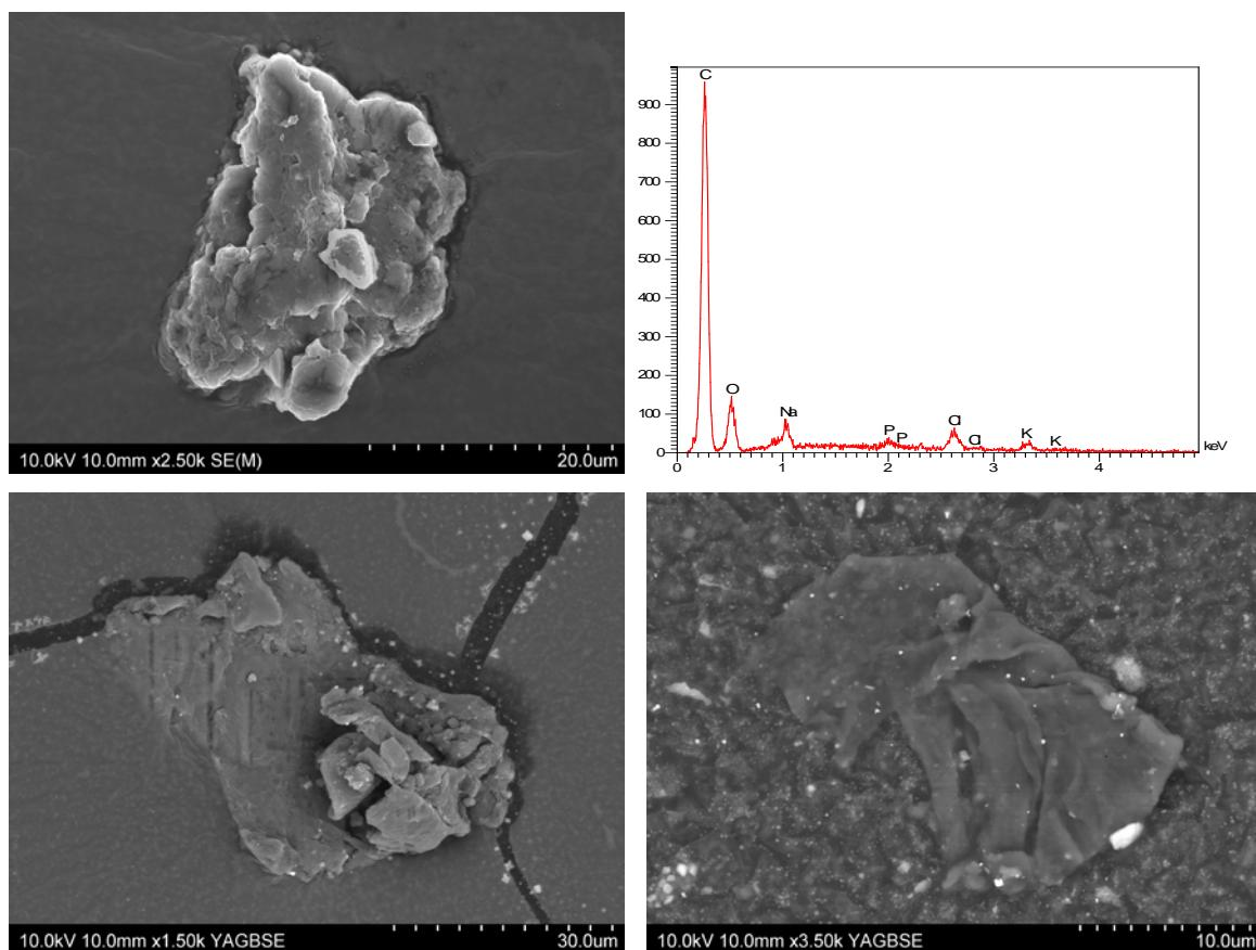
**Figure 21: SEM picture and spectrum (Au-Pd metallation) of carbonaceous residue obtained after HCl demineralization of the mixture fluoranthene/limestone oxidized 6 months.**
