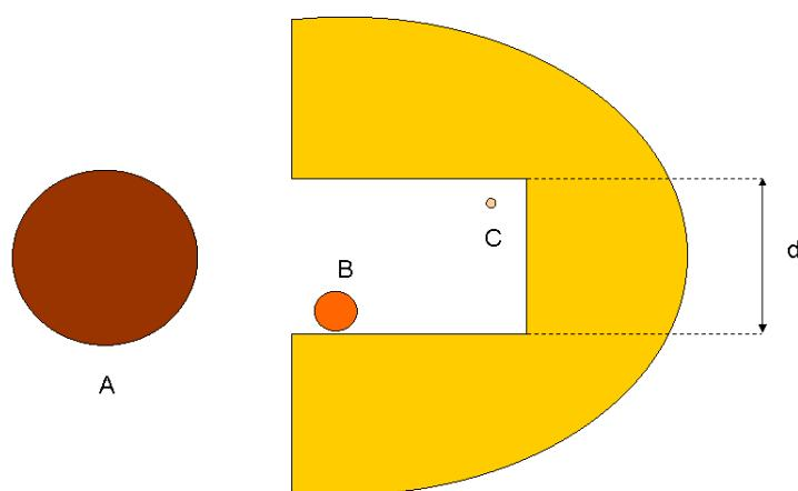
**Figure 2 :** Size exclusion mechanism, according to the ratio  $2R_h/d$ , there are 3 possibilities, a complete exclusion (A), a selective exclusion (B) or complete permeation (C) of the macromolecule.
