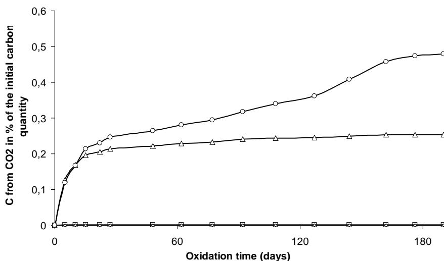
**Figure 12:**  $\text{CO}_2$  production during oxidation experiments at  $100^\circ\text{C}$  for pure fluoranthene ( $\diamond$ ), for the mixtures fluoranthene/silica ( $\square$ ), fluoranthene/clay ( $\circ$ ) and fluoranthene/calcite ( $\Delta$ ).
