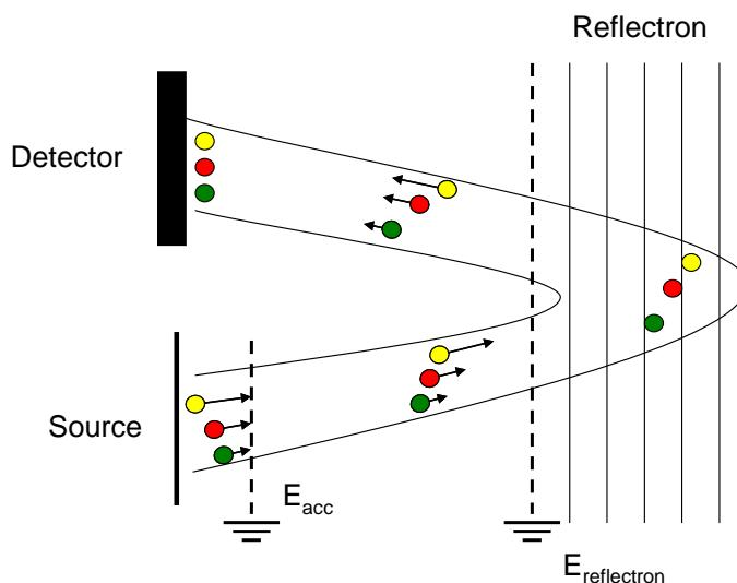
**Figure 23: Principle of the use of reflectron in TOF analyzer**
