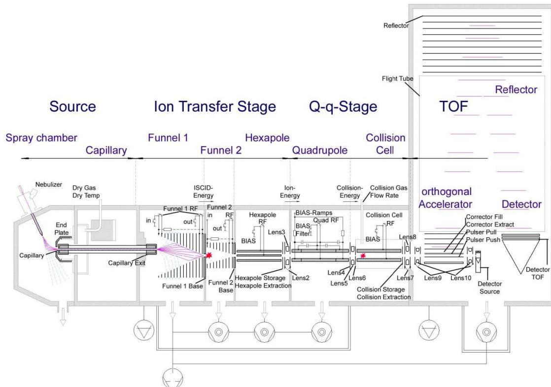
**Figure 24:** Schematic of orthogonal injection Q-TOF (reproduced from Bruker MicrOTOF<sub>Q</sub> user manual).
