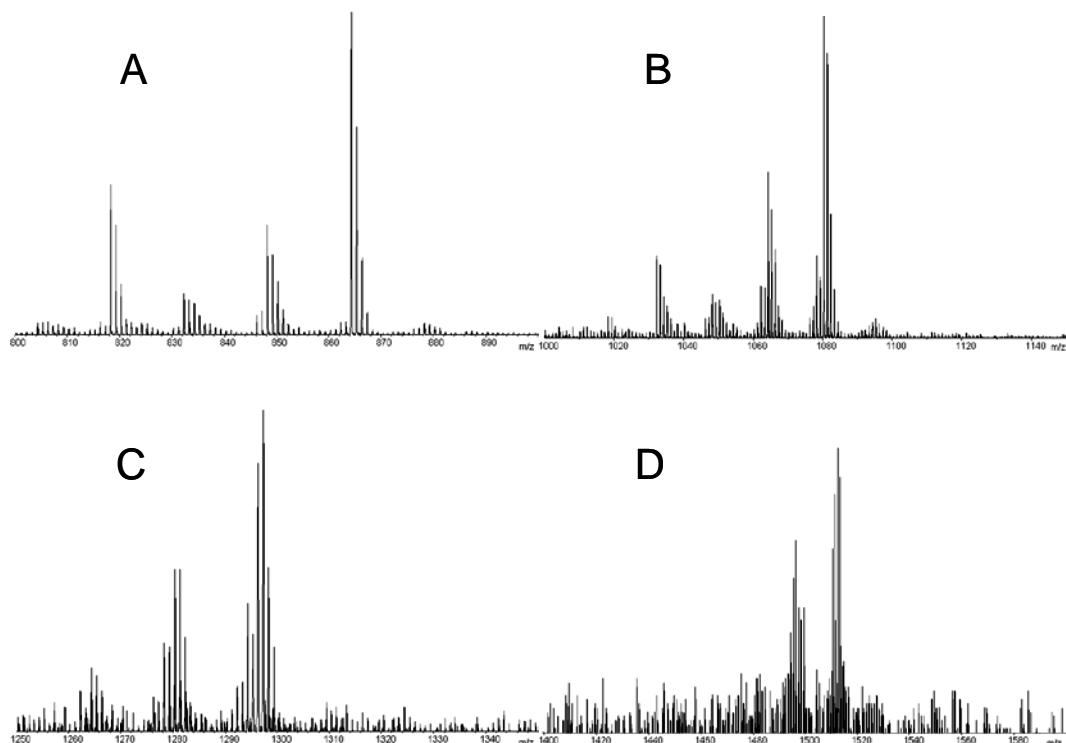
**Figure 7:** APPI+ mass spectra of the oxy-PAH sample using GPC Mixed E column. Spectrum A: from 800 to 900 Da, spectrum B: from 1000 to 1150 Da, spectrum C: from 1250 to 1300 Da, spectrum D: from 1250 to 1300 Da.
