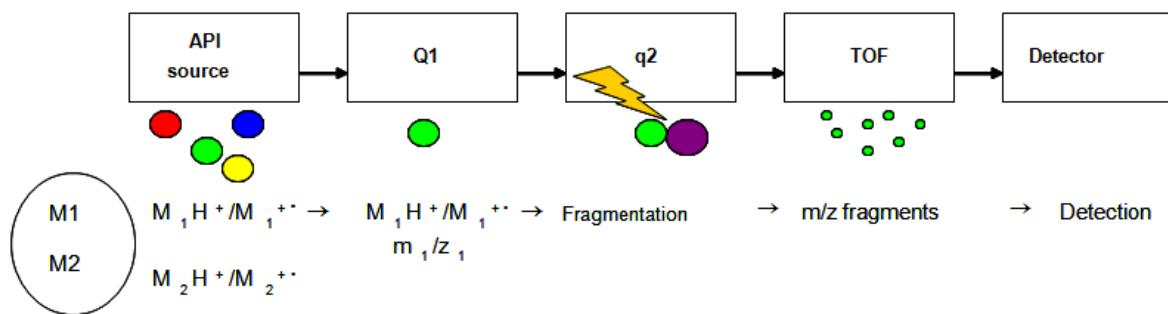
**Figure 11: Simplified MS/MS experiments (case of Q-TOF mass analyzer).**
