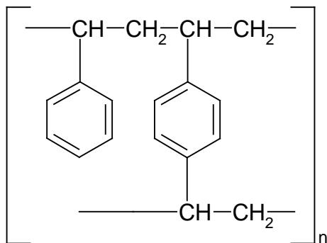
**Figure 6:** Structural formula of the styrene divinyl benzene monomer.
