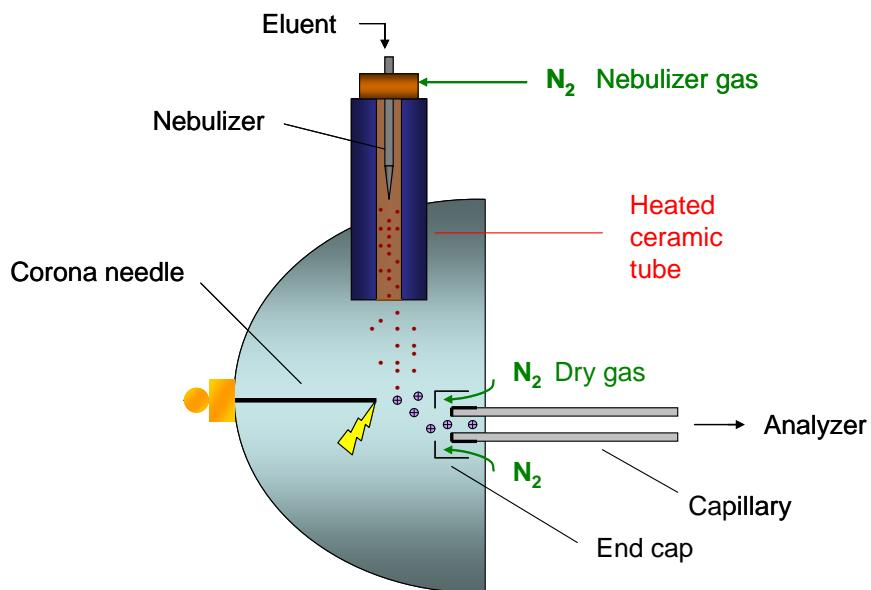
Figure 16 : Schematic of an APCI source.
