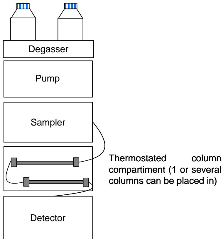
**Figure 3 : Schematic representation of a classical SEC system.**
