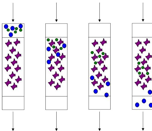
**Figure 1:** Principle scheme of SEC chromatography for 2 different molecules. After the sample injection the molecule will evaluate differently according to their molecular mass, the bigger ones will pass through the column faster than the small ones.
