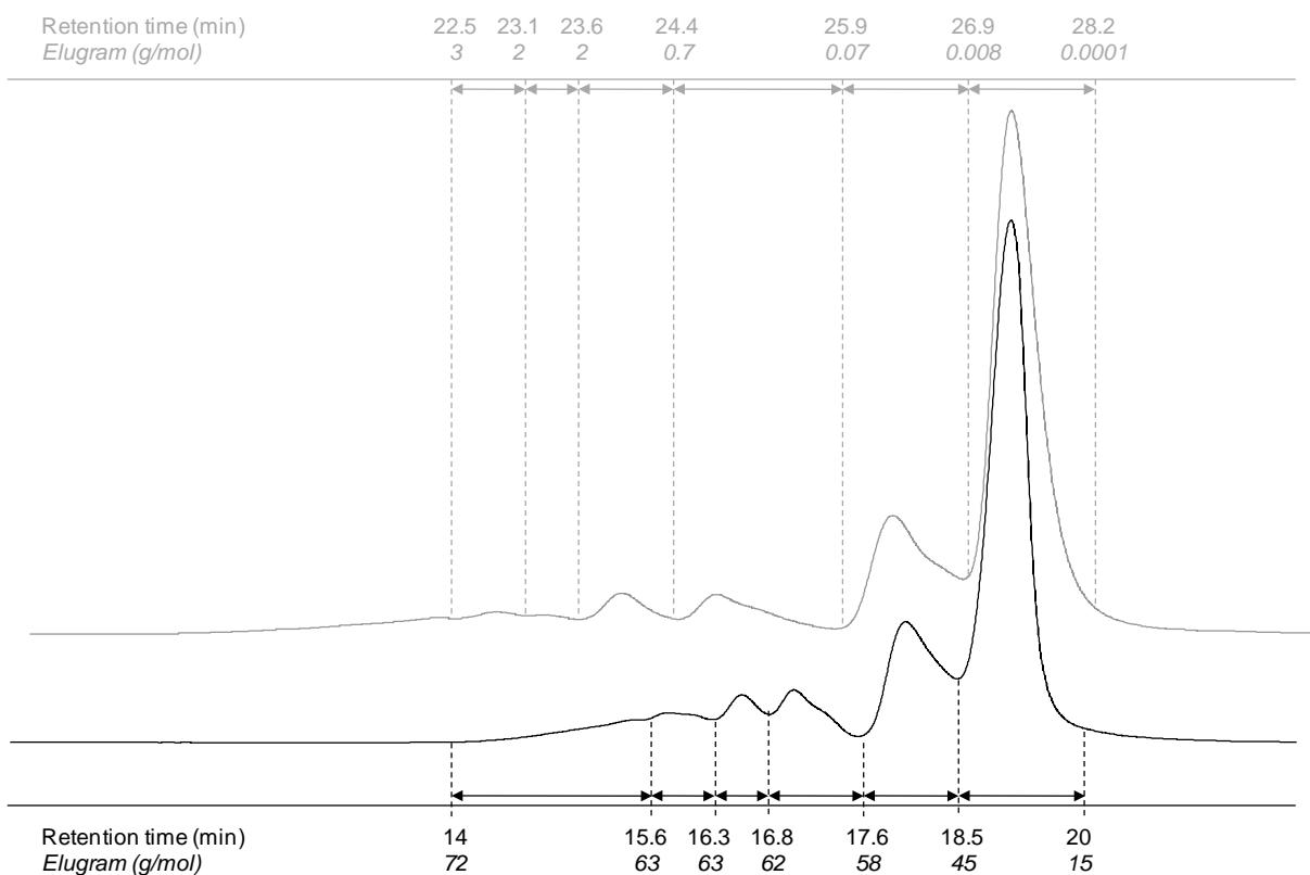
**Figure 8: UV chromatograms of the oxy-PAH mixture at 300nm, using GPC Mixed E column (black line); using a combination of GPC Mixed E + HR columns (grey line) with respective molecular mass calibration using polystyrene standards.**
