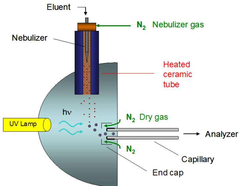
Figure 17 : Schematic of an APPI source
