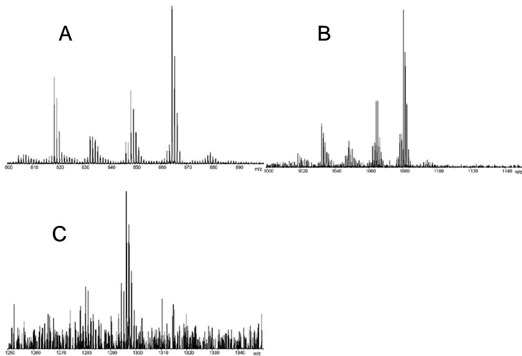
**Figure 5: APPI+ mass spectra of the oxy-PAH sample using GPC Mixed E column. Spectrum A: from 800 to 900 Da, spectrum B: from 1000 to 1150 Da, spectrum C: from 1250 to 1300 Da.**
