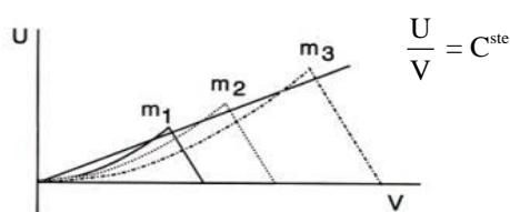
**Figure 21:** Stability area A ( $U=f(V)$ ) for different mass ions ( $m_1 < m_2 < m_3$ )
