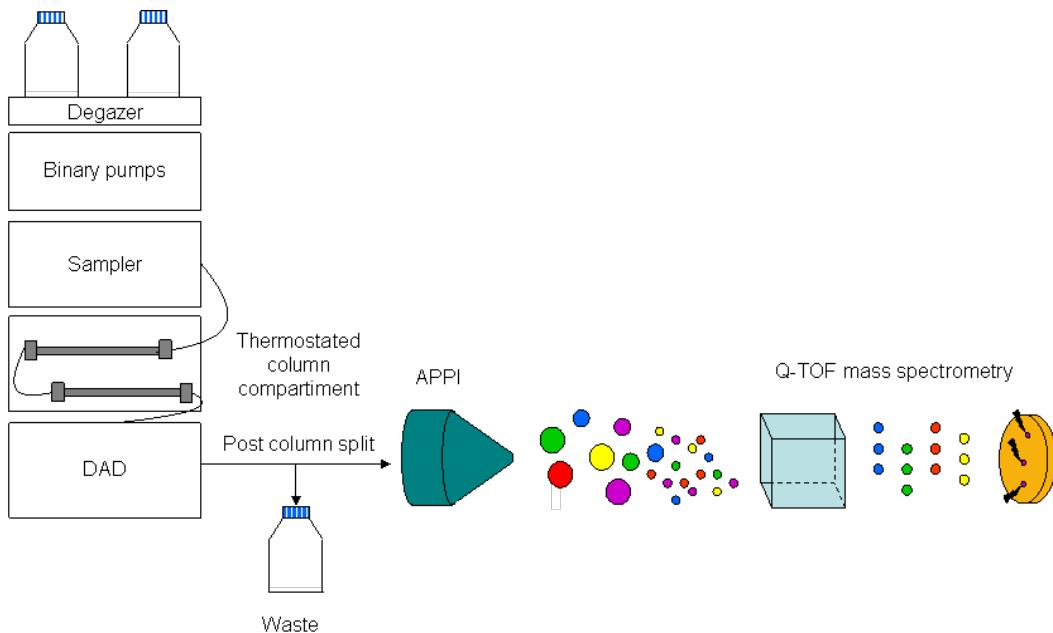
**figure 1: Composition of the analytical system involving the SEC and the APPI-Q-TOF mass spectrometry**
