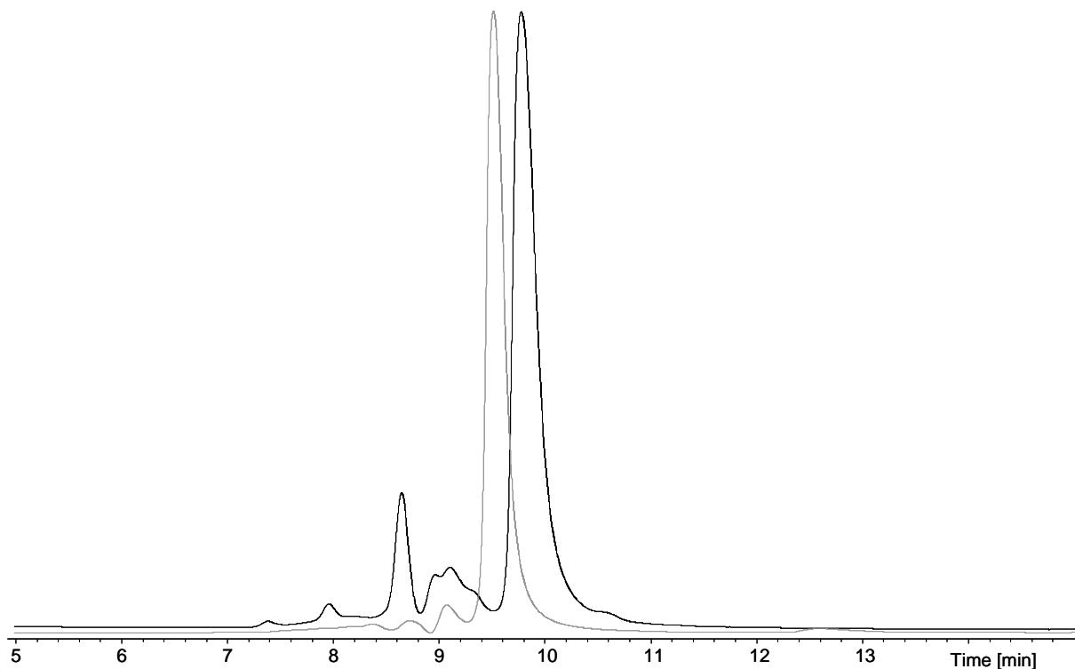
**Figure 2:** Size Exclusion Chromatograms obtained on Mixed-E column for the oxy-PAH sample using respectively tetrahydrofuran (-) and chloroform (-) as mobile phases. Agilent HPLC 1100 series chromatograph with UV detection (300nm).
