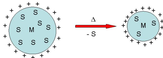
**Figure 13: Evaporation scheme of the solvent from charged droplet (M is the analyte and S is the solvent)**
