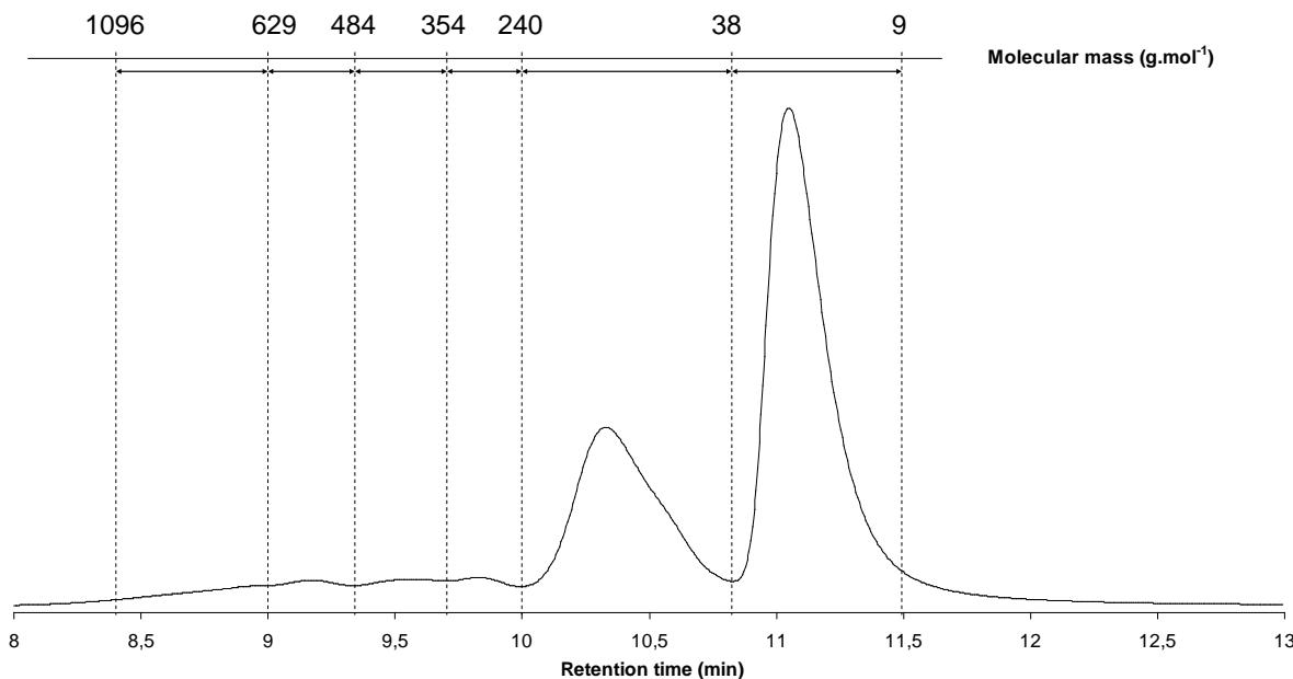
**Figure 3: SEC molecular mass distribution of the oxy-PAH mixture (Mixed-E column, THF mobile phase at 1mL.min<sup>-1</sup>, UV detection at 300nm) according to polystyrene standards calibration. The highest peak corresponds to fluoranthene (m/z 202) and the second highest to PAHs and Oxy-PAHs of m/z ranging from 400 to 500 as determined by direct infusion APPI-QTOF**
