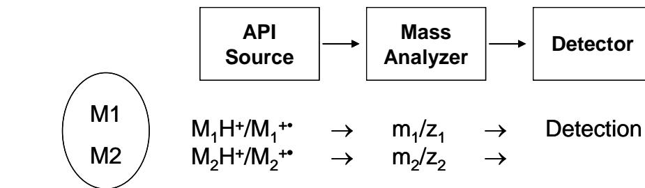
**Figure 10: Simplified MS experiments.**
