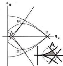
**Figure 20:** Stability diagram,  $a_u=f(u)$  for an ion with a specific mass  $m$
