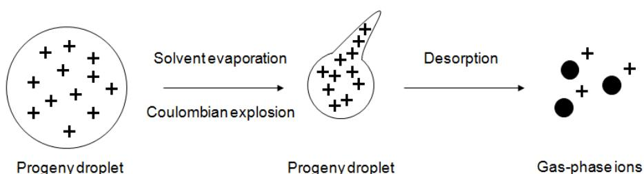
**Figure 15: Ion evaporation model.**
