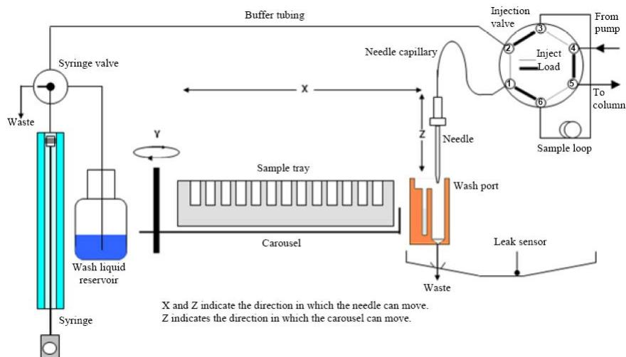
**Figure 4:** Schematic representation of the sampler (Dionex ACC300), reproduced from Dionex operating manual.
