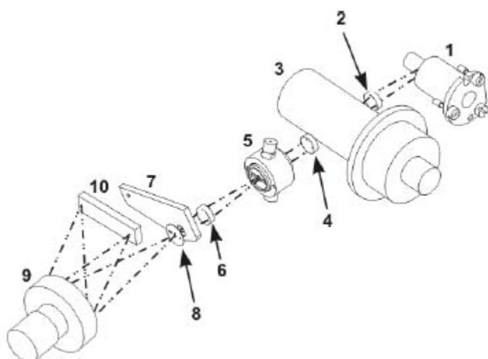
Figure 7: optical system for Dionex DAD3000, reproduced from Dionex user manual.
