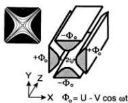
**Figure 19 : Quadrupole with hyperbolic rods**
