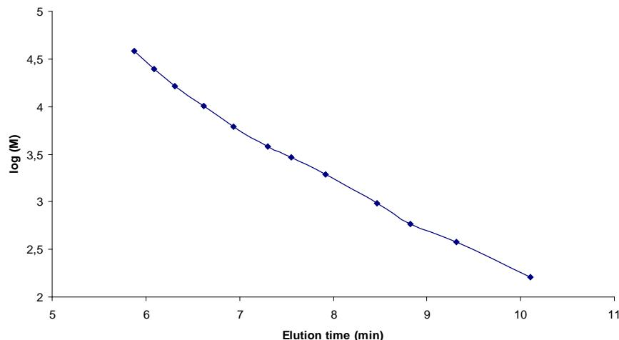
**Figure 8: Example of classical calibration using polystyrenes as standards using THF as eluant at 25°C on Mixed E GPC column.**
