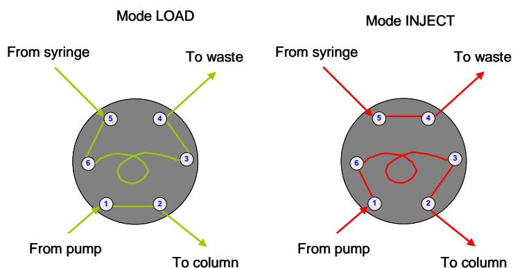
**Figure 5:** Representation of the 2 operating modes (load and inject) of the 6 way valve.
