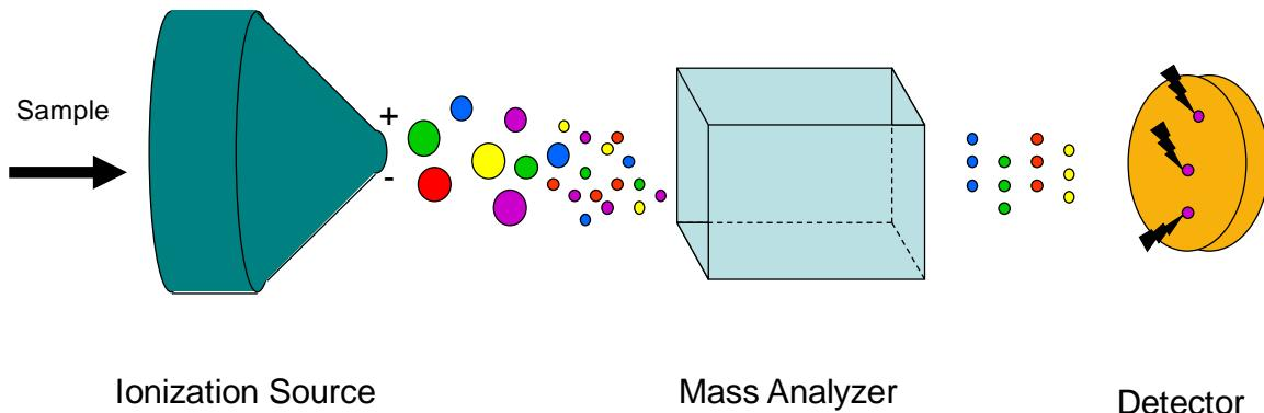
**Figure 9 : Principal scheme of mass spectrometry instrumentation.**
