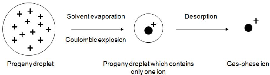
**Figure 14: Residual charge model.**
