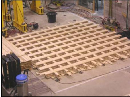
*Figure 3. The suspended floor, 4 x 4 m<sup>2</sup> and 216 mm thickness, built of welded spruce slat. M. Properzi *et al.* (2005) [35].*
