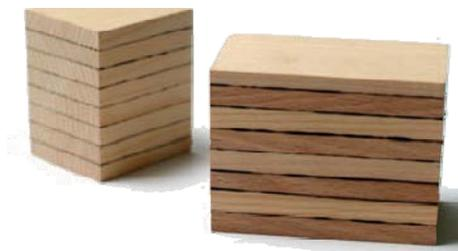
Figure 2. Multilayered wood laminate, built of eight alternating layers of spruce and beech boards; beech shows a darker color. B. Stamm et al. (2005) [34].
