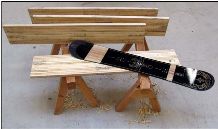
Figure 5. Welded blocks of *Populus sp* used in the manufacture of snowboard's cores. C. Ganne-Chedeville, (2006) [31].
