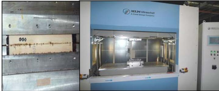
Figure 16 : linear vibration welding machine (LVW 2061 Mecasonic made in Annemasse, France), M.Vaziri et al. 2010 [46, paper II].
