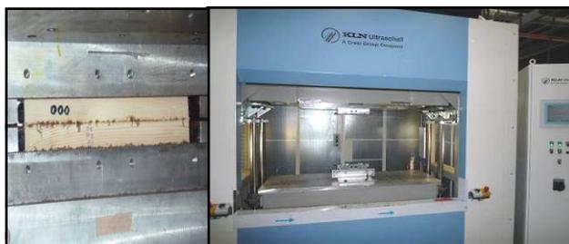
*Fig 1. Linear vibration welding machine LVW 2061 Mecasonic made in Annemasse, France.*
