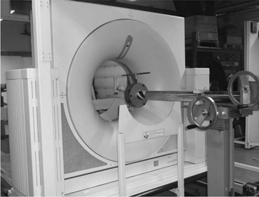
**Figure 2.** CT-scanner and scanning of a sample taken out of the water.
