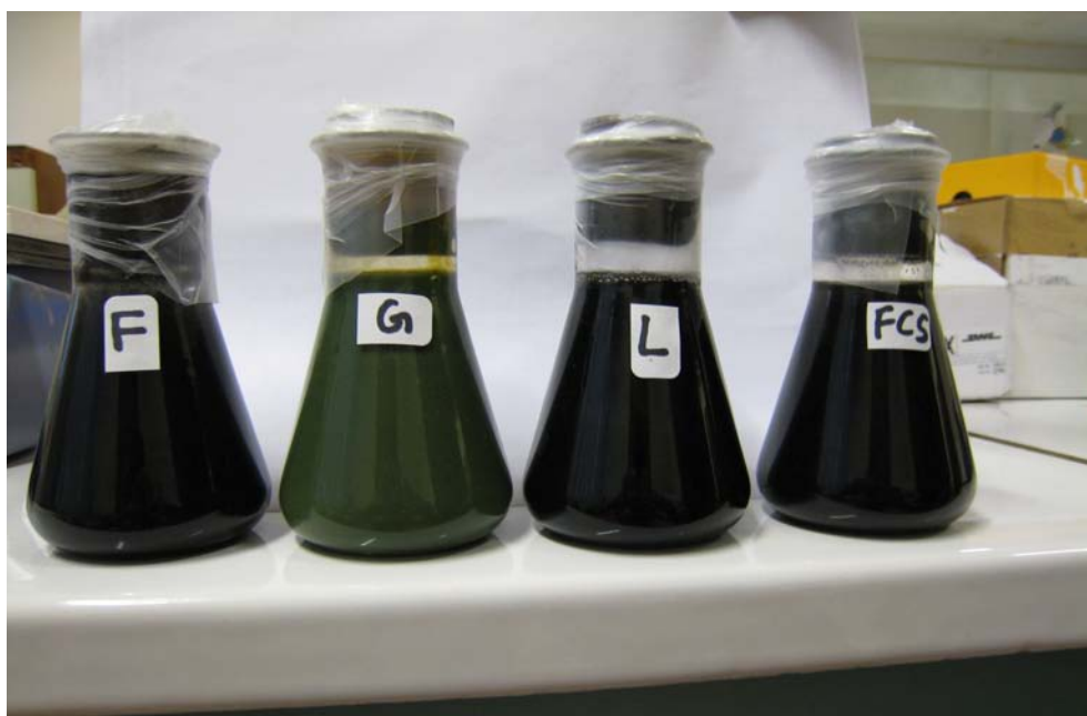
Figure 1.1: Transformations of ferrihydrite (F), goethite (G), lepidocrocite (L) and ferrihydrite rich sand (FRS) into magnetite performed in batch slurry systems. Difference in transformation reactivity is prominent for G as shown by its color.
