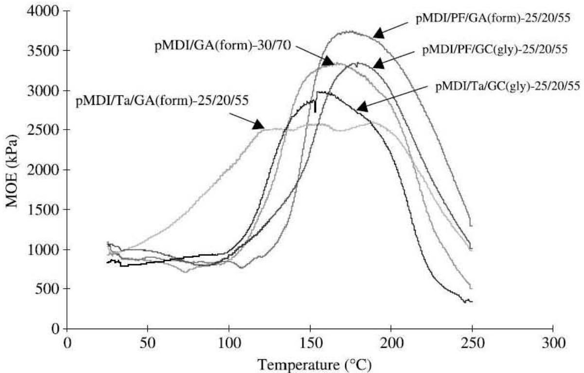
**Figure 1.** Modulus of elasticity (MOE) variation as a function of temperature obtained by thermomechanical analysis (TMA) of different gluten protein-formaldehyde and gluten protein-glyoxal adhesive formulations. Gluten protein hydrolysate produced chemically (G). GA(form) = gluten reacted with formaldehyde. GC(gly) = gluten reacted with glyoxal. Ta = tannin.
