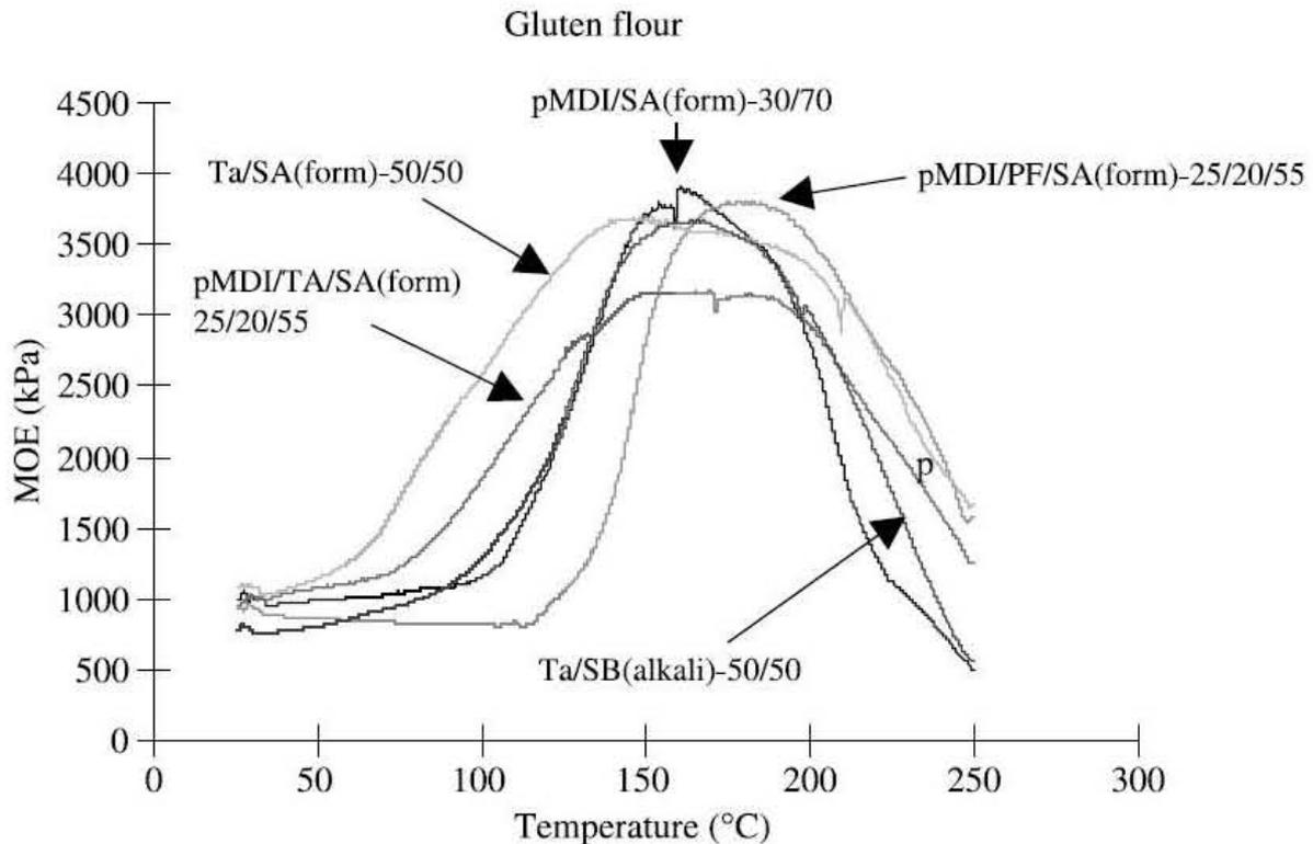
**Figure 3.** Modulus of elasticity (MOE) variation as a function of temperature obtained by thermomechanical analysis (TMA) of different gluten protein-formaldehyde and gluten protein-glyoxal adhesive formulations. Gluten flour (S). SA(form) = gluten reacted with formaldehyde. SB(alkali) = gluten pretreated with alkali. Ta = tannin.
