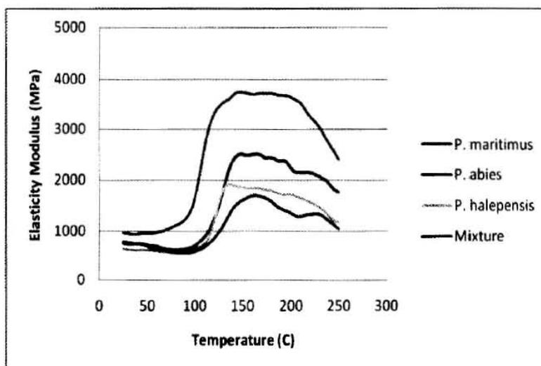
**Figure 4.** Thermomechanical test comparison by elasticity's modulus (MOE).
