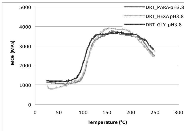
Figure 11: Thermomechanical analysis (TMA) of DRT maritime pine tannin at pH = 3.8 with various hardeners.
