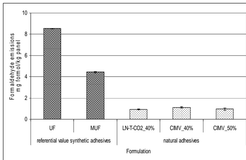
Figure N° 7: Formaldehyde emissions by EN-717-3 standard method.
