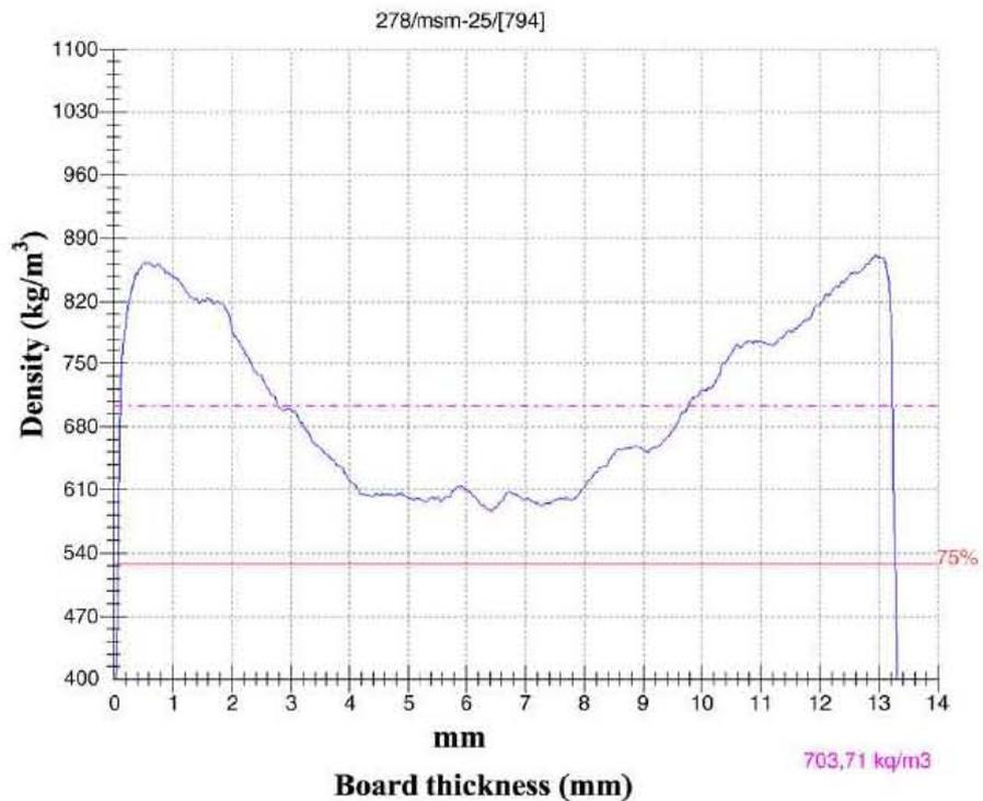
The panel density profiles were done on all the specimens tested for internal bond, before destructive testing, by using a Grecon Da-X (Greten, Germany) density profiler.
