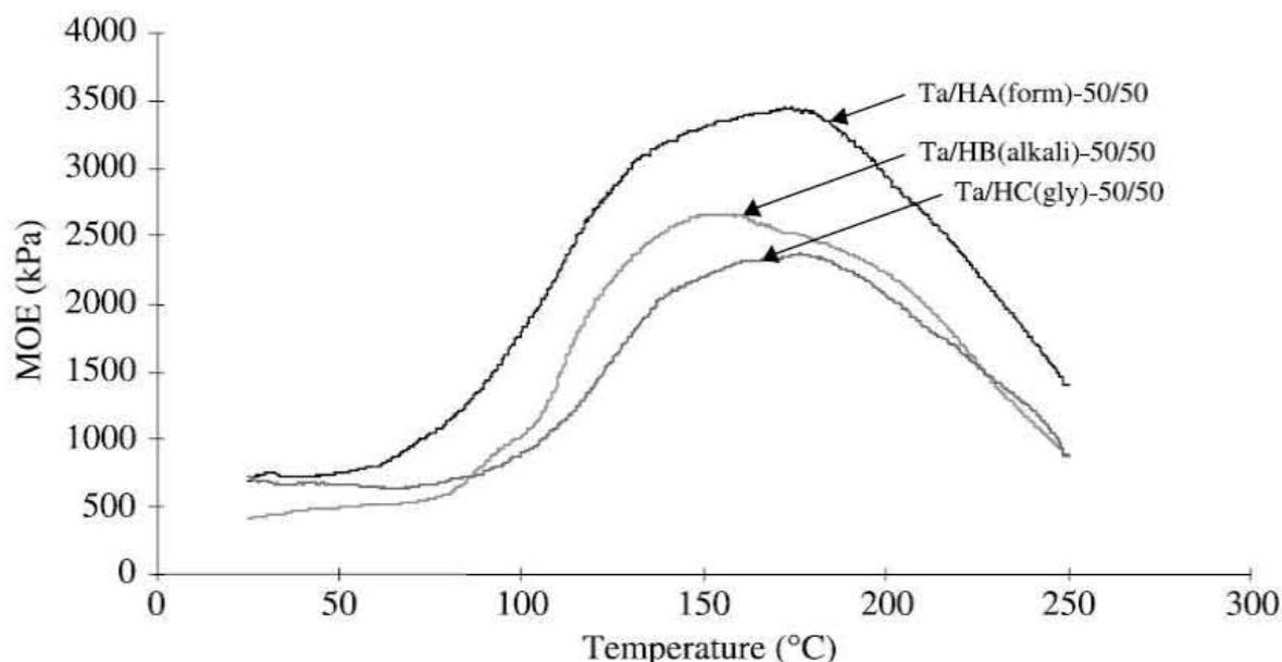
**Figure 2.** Modulus of elasticity (MOE) variation as a function of temperature obtained by thermomechanical analysis (TMA) of different gluten protein-formaldehyde and gluten protein-glyoxal adhesive formulations. Gluten protein hydrolysate produced enzymatically (H). HA(form) = gluten reacted with formaldehyde. HB(alkali) = gluten pretreated with alkali. HC(gly) = gluten reacted with glyoxal. Ta = tannin.
