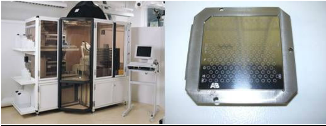
Figure 16 : Ettan Spot Handling Workstation et cible MALDI TOF (source : http://www.gelifesciences.com/ et http://www.appliedbiosystems.com/ respectivement)
