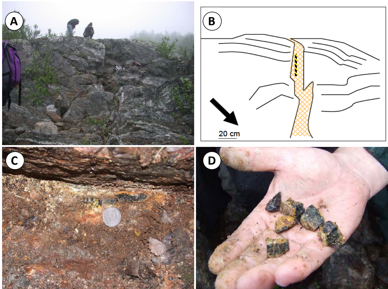
Figure 2.21. A. Photograph and B. Scheme of outcrop Litsa_111 showing a subvertical, NE-striking, 20 cm wide, quartzfeldspar± muscovite vein (outcropping over 22m), which crosscuts NW-striking biotite-rich gneisses. A pitchblende vein, <1 cm thick, NE striking, has outcrops within the felsic dyke over 1.5 m (black and yellow line). Pitchblende vein of the Litsevskoe ore-showing. C. Pitchblende vein within quartz-muscovite vein; D. Pitchblende with hexavalent uranium minerals [sample 65.1].
