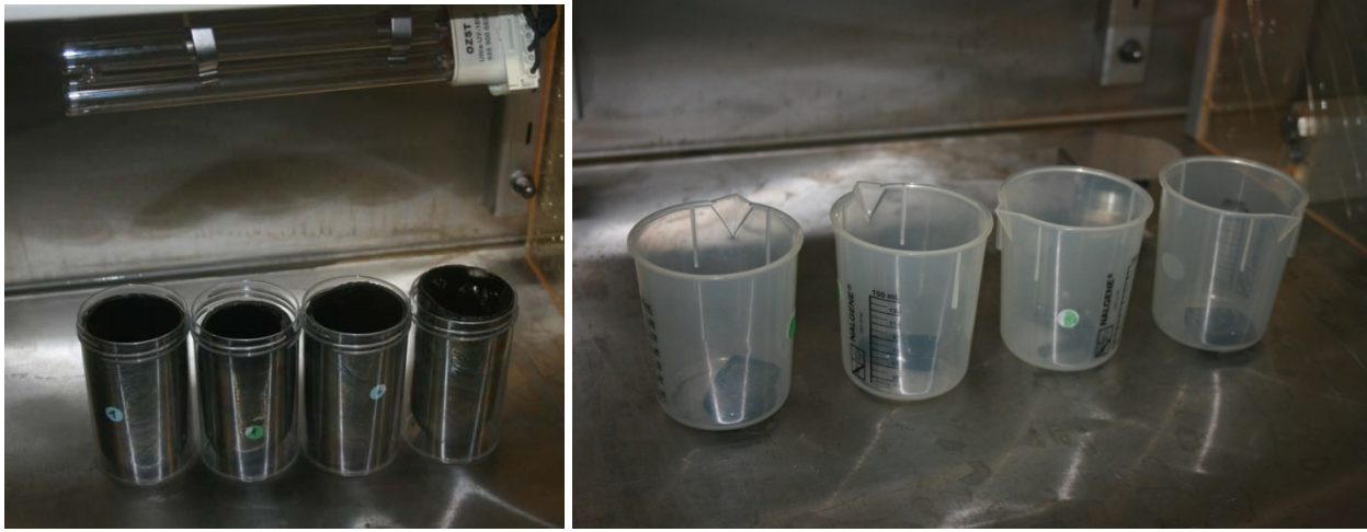
Figure 2: a) Basaltic glass beakers included in experiments with UVC irradiations. b) Basaltic glass bars included in Nalgène beaker for experiments without UVC irradiations.
