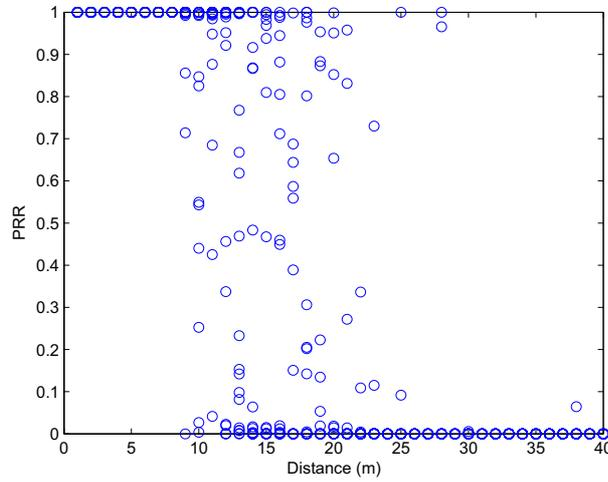
FIGURE 2.3: Analytical PRR to distance, obtained from equation (2.18) and (2.16),  $P_t = -5\text{dB}$ ,  $\eta = 3$ ,  $\sigma = 3.3$ ,  $f = 50$  bytes,  $h = 2$  bytes.
