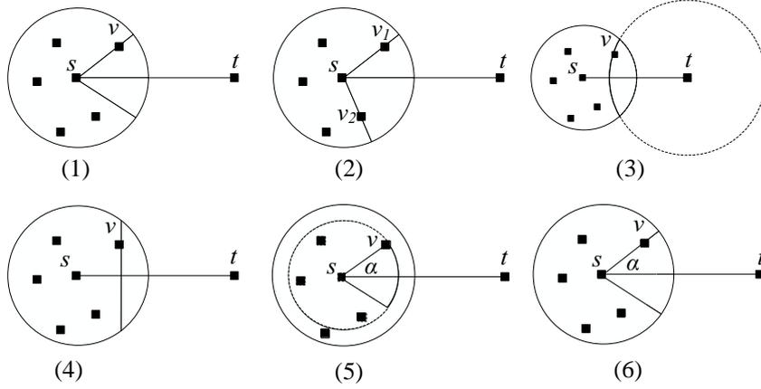
FIGURE 4.1: Various forwarding methods for geographic routing.
