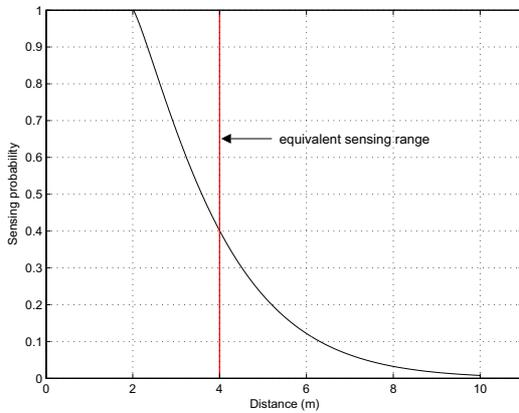
FIGURE 3.9: Sensing model, indicating equivalent sensing range under disk model.
