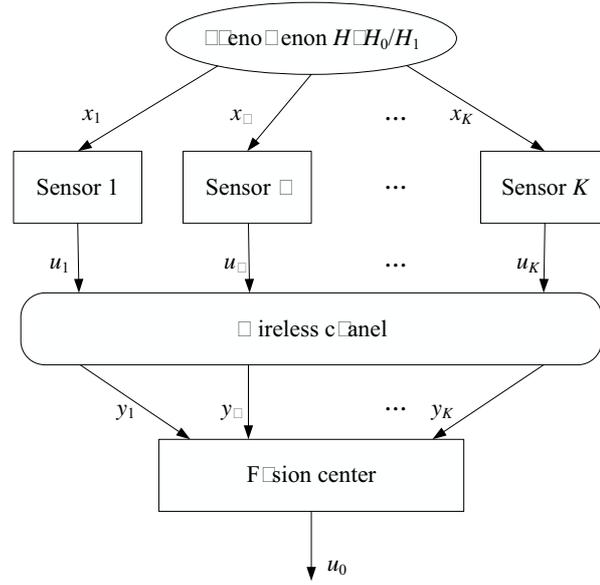
FIGURE 5.1: Paralleled distributed detection system under fading channel
