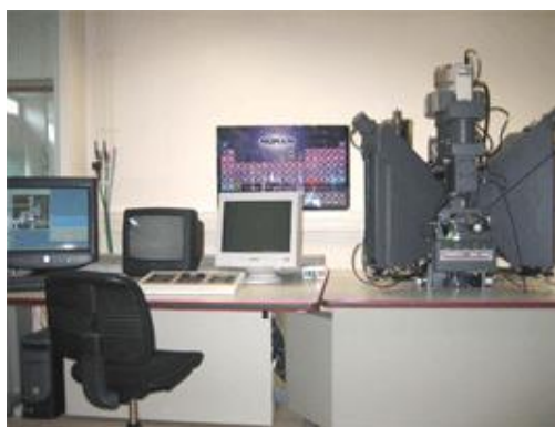
Photo II.4 - Microsonde CAMECA SX100
