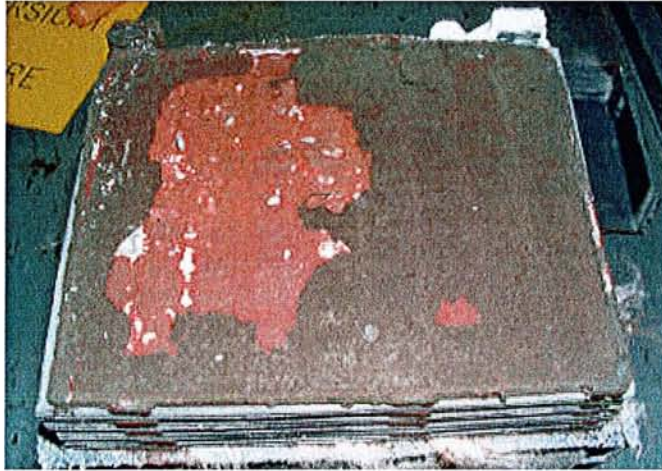
Figure 94: Surface of a positive plate at the opening of a battery after cycling with phosphoric acid
