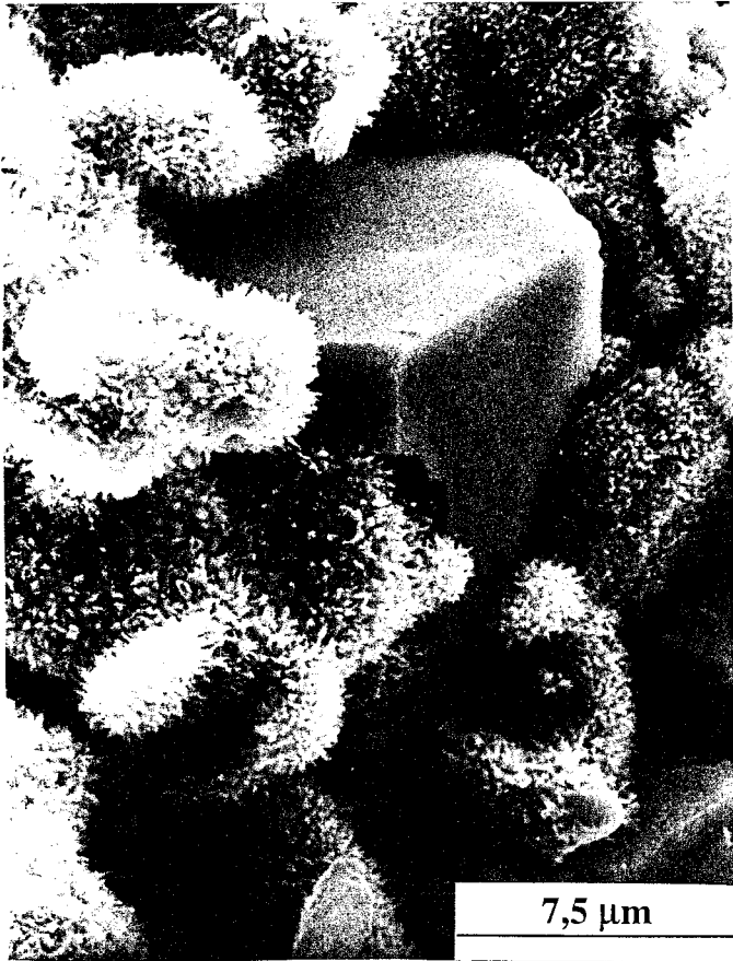
PHOTO N°12 : Interactions C_xS_yH_z - \overline{CC} ( C_3S-15\% \overline{CC} 1 j MH)
