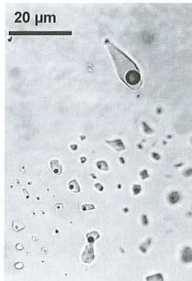
Figure B-10: Photomicrograph of petroleum and aqueous contemporaneous fluid inclusions in fluorite crystal from the Cave-in-Rock MVT deposit, fluorite-Pb-Zn district, southern Illinois, USA.
