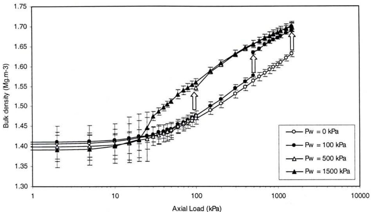
**Figure 4: Hydrocollapse curves for 25-35 cm depth soil sample.**
