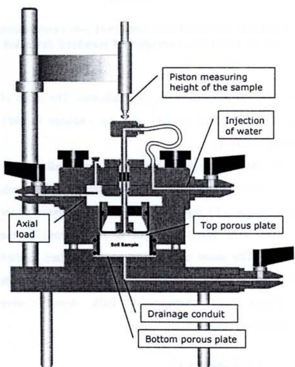
Figure 1: Oedometer apparatus
