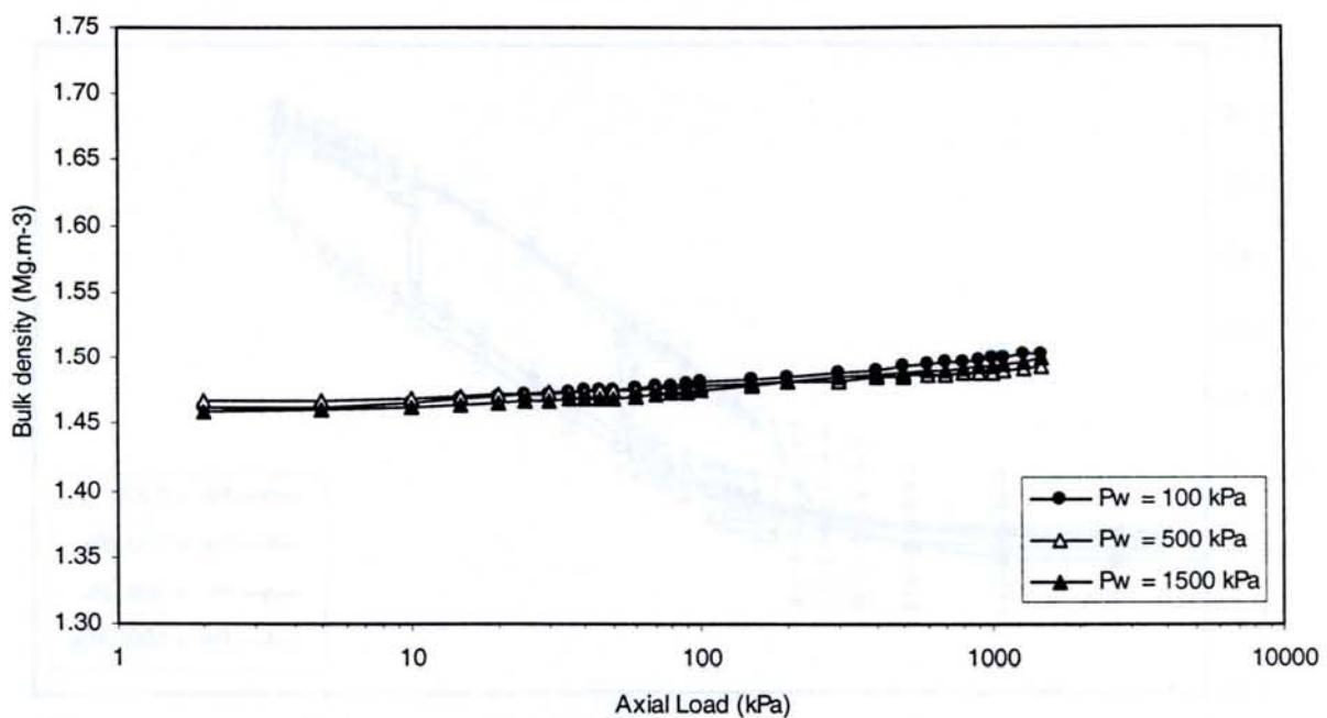
**Figure 3: Hydrocollapse curves for pure sand material.**
