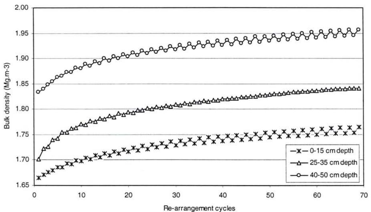
Figure 6: Bulk density during re-arrangement cycles (0-1500 kPa).
