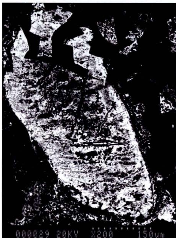
Fig. 3.38. BSEM image of a Ti-U oxide (detrital brannerite ?) in the mineralized Priozersk sandstones – (DDH-680-125 m (Karku deposit area, ore zone III). Photomicrograph scale = 150 \mu m
