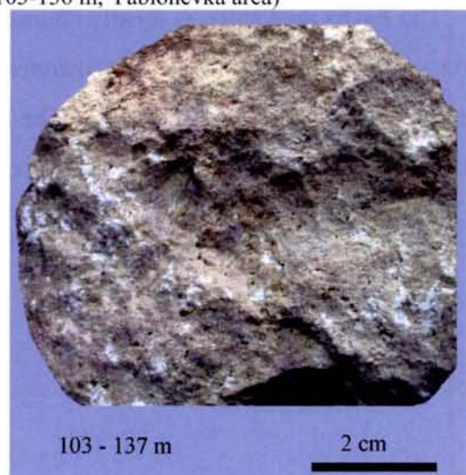
Fig. 3.8. Stromatolite-like dolomitic rocks within the essentially clastic sequences (sample DDH-103-137 m, Yablonevka area)
