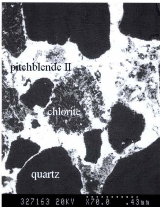
Fig. 3.34. BSEM image of corroded quartz crystals in a cement composed of pitchblende II and chlorite with sulphides. Sample DDH-671-132 m (Karku deposit area, ore zone III), photomicrograph scale = 43 mm
