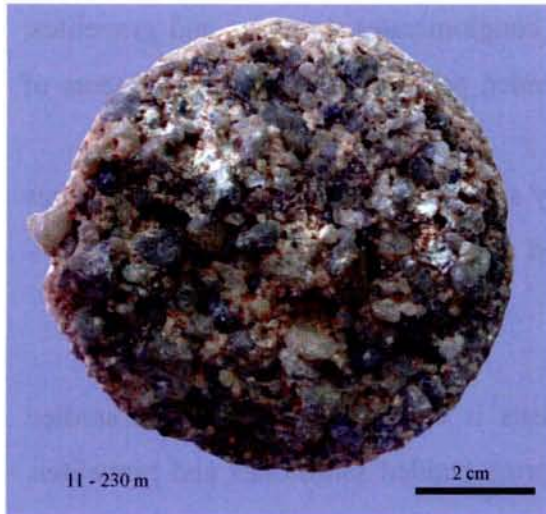
Fig. 3.10. Quartz-feldspar small-pebbled conglomerate of the Pasha suite (sample DDH-11-230 m, Pasha area)
