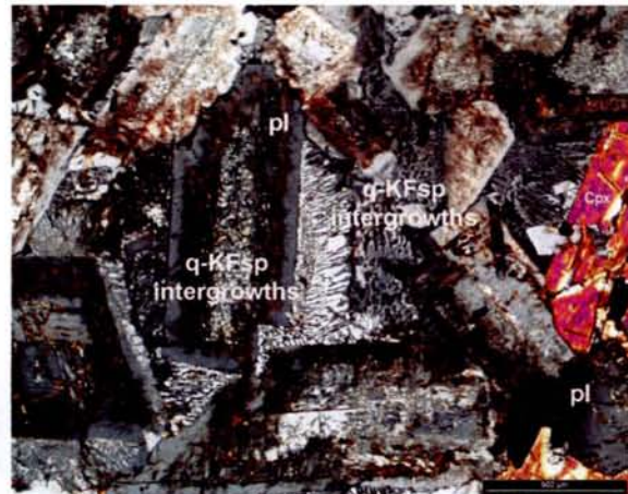
B. Quartz – orthoclase intergrowths in and between plagioclase (sample 2085). Crossed nicols, line scale – 0.5 mm.
