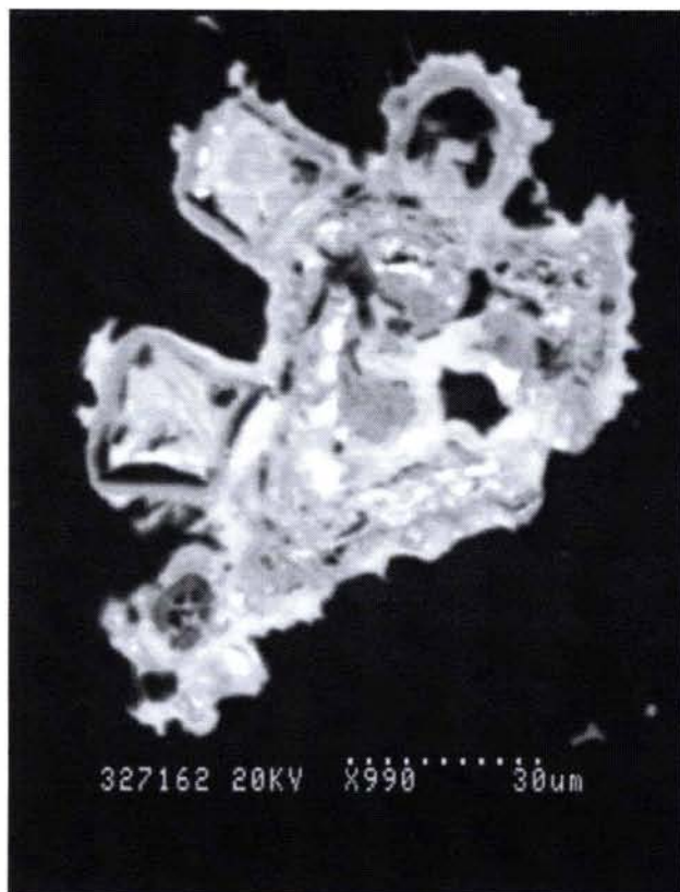
Fig. 3.42. BSEM image of skeletal crystal of Ni – Co arsenides (DDH-384-144, Karku deposit area, ore zone I), photomicrograph scale = 30 \mu\text{m}
