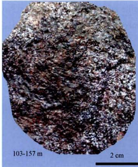
Fig. 2.51. Regolithized quartz-biotite feldspar gneiss in the vicinity of the unconformity surface (Yablonevka area, DDH-103-157 m)
