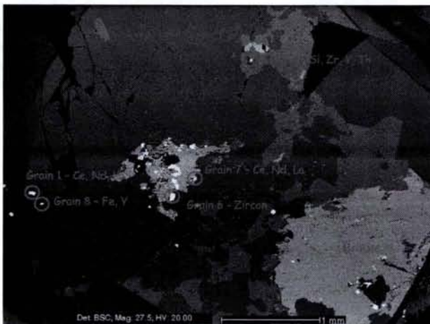
Fig. 2.89. Abundant REE-bearing accessory minerals included in biotite in the even-grained biotite granite (sample 5-04-01, Pitkyaranta area). BSEM image, photomicrograph scale – 1 mm
