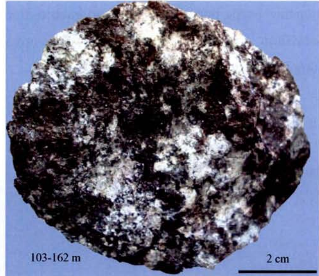
Fig. 2.52. Slightly regolithized quartz-biotite feldspar gneiss at 5 meters from the unconformity surface (Yablonevka area, DDH-103-162 m)
