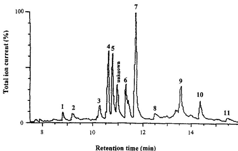
Figure 1. GC/EI-MS of a non-polar TLC fraction (zone III;  $R_f$  0.7) of DNPH carbonyls resulting from oxidized linolenic acid: 1: pentanone; 2: butanal; 3: hexanal (*syn*); 4: hexanal (*anti*); 5: 2-hexenal; 6: 3-hexenal (*syn*); 7: 3-hexenal (*anti*); 8: hexadienal; 9: heptadienal; 10: octadienal; 11: nonadienal.
