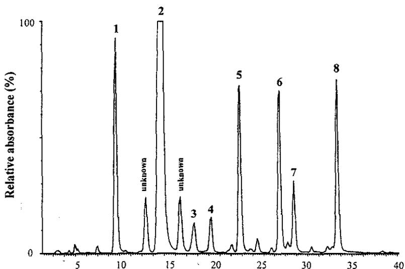
Figure 2. DNPH derivatives of aldehydes identified using LC/ESI-MS and monitored by UV detection ( $\lambda = 360$  nm) in a non-polar TLC fraction (zone III;  $R_f$  0.6) of oxidized linolenic acid: 1: acetaldehyde; 2: propanal; 3: butanal; 4: butanal; 5: pentanal; 6: hexenal; 7: heptadienal; 8: nonadienal.
