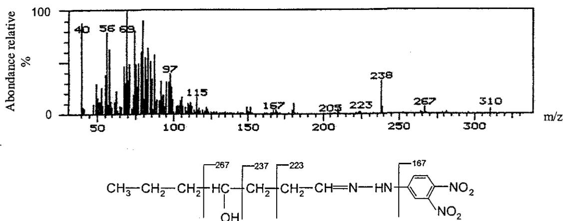
Figure 26 : Spectre EI du 4-hydroxyheptanal-DNPH ( $M=310$ ).
