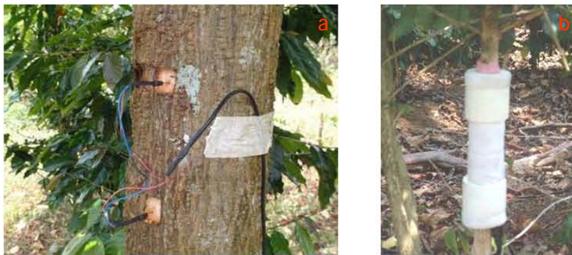
Photography 7. Detailed views of the measurements of tree sap flow with “Granier” sensors (a) and coffee sap flow with Dynamax gauges (b) on the research station of CICAPE, San Pedro de Barva, Heredia, Costa Rica.
