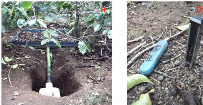
Photography 8. Detailed views of the measurements of water runoff (a) and soil water content with TDR (b) on the research station of CICAPE, San Pedro de Barva, Heredia, Costa Rica.
