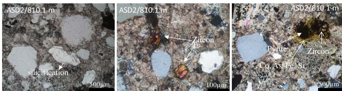
Figure III. 9: ASD2 (9312) drill hole: corroded grains of quartz with weak silicifications, carbonated and sericitic matrix. Accessory minerals are abundant (ex. zircon).
