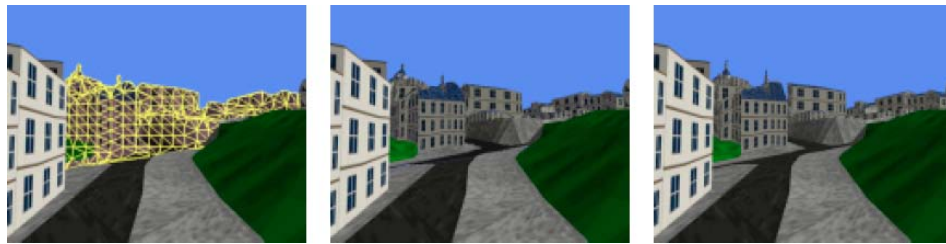
Figure 4.23: Results of Sillion et al. work [SDB97]. Left : impostor mesh; center : the composed image at about 15 fps; Right : the original image at 2 fps.
