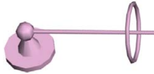
Figure 9.13: This model portion is composed by two cylinders, one complete torus, one complete cone and one sphere. The topological reverse engineering can find the cylinders and the torus (actually, two half tori since we search for torus sections with up to 180 degrees). In order to detect complete cones and spheres the numerical fitting approach is required.
