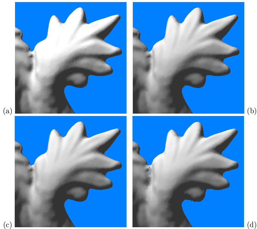
Figure 8.7: (a)Original dragon model with 800K triangles. (b)Dragon rendering with 512 \times 512 geometry textures. (c)Dragon rendering with 256 \times 256 geometry textures. (d)Dragon rendering with 128 \times 128 geometry textures.
