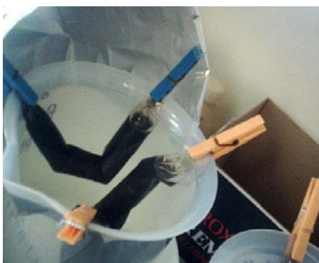
Figure 1.2. Dialysis membranes containing a solution of a mixture of synthetic fulvic acids.
