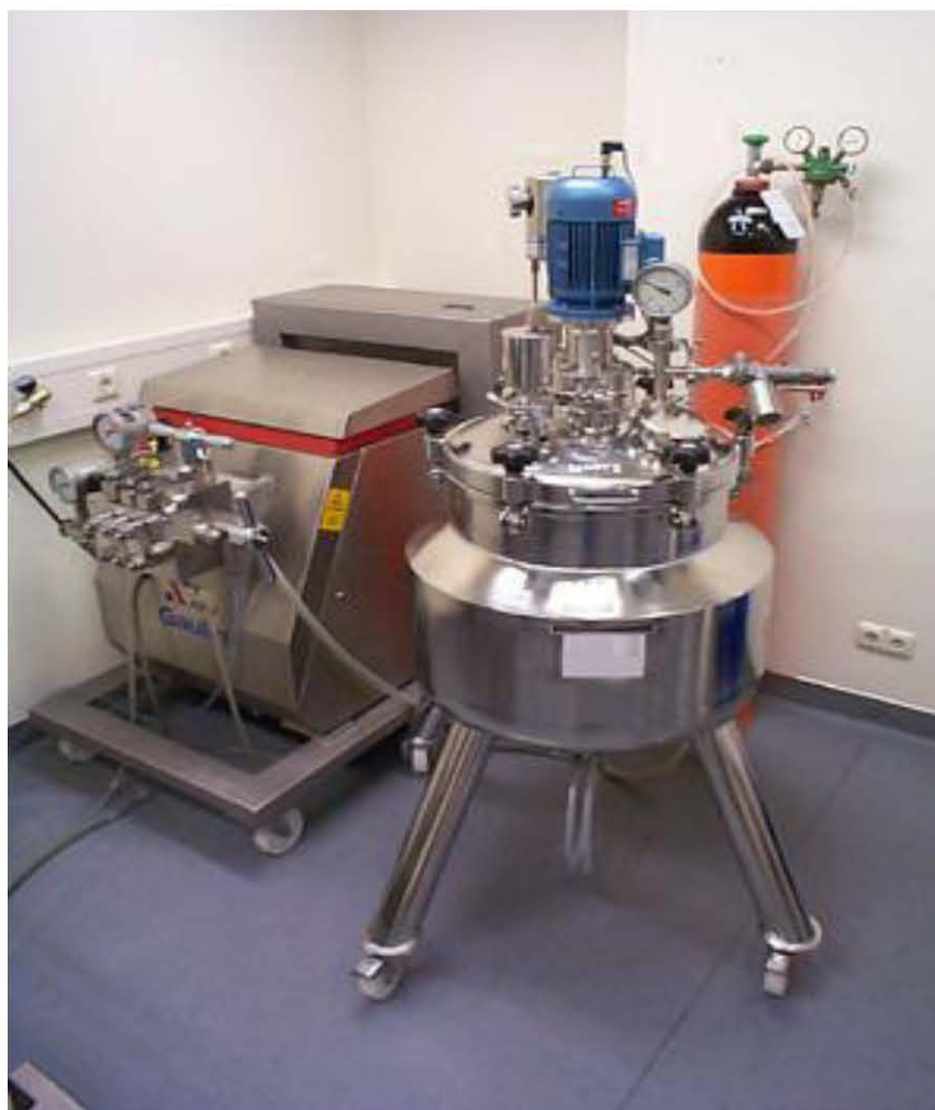
Fig. 2.10: A typical arrangement for a Gaulin 5.5 with attached product container (right)
