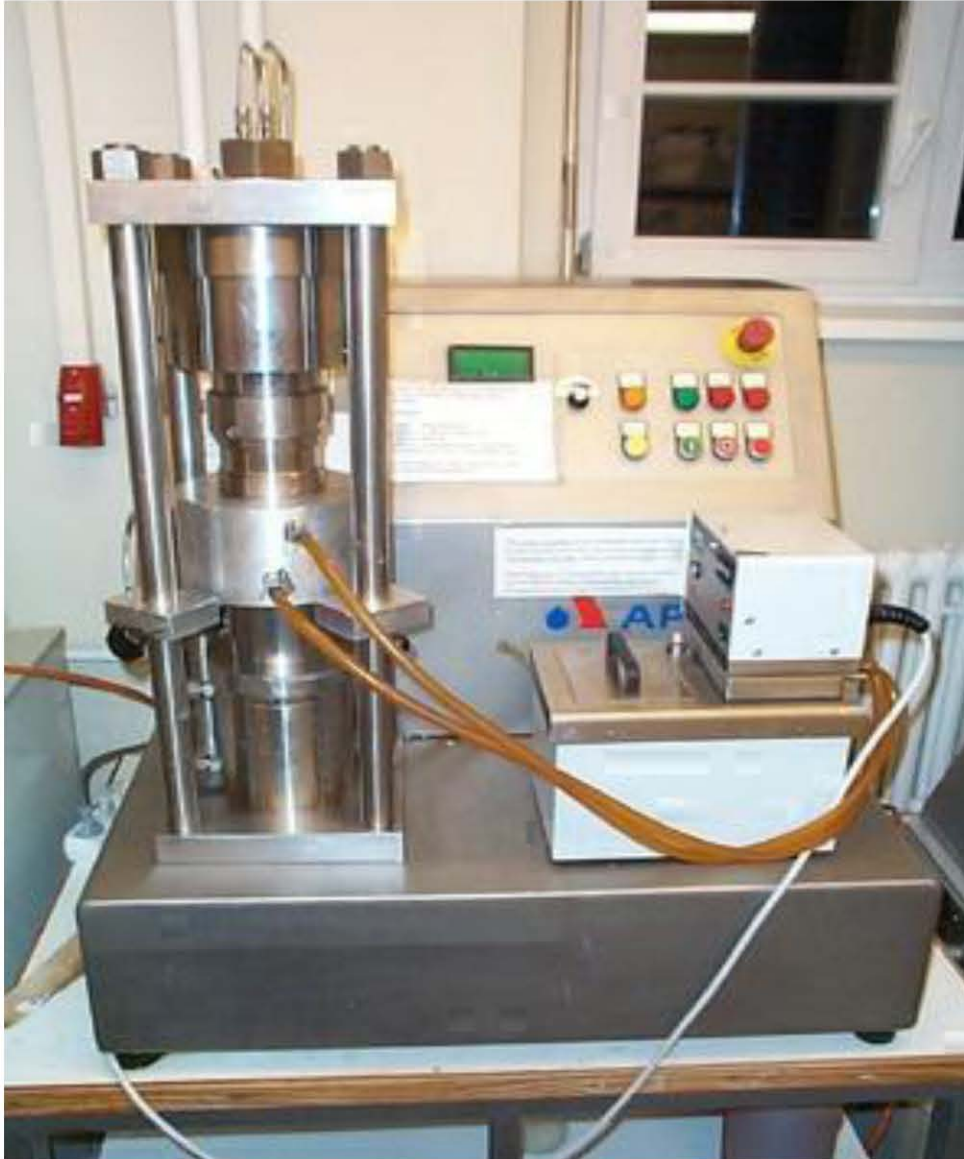
Fig. 2.9: LAB 40 homogenizer with temperature control unit
