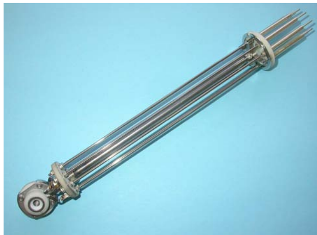
Figure 4.17. Photograph of the entire probe head before insertion into the CFC housing. The length of the probe from the centre of the tunnel to the end of the pins is 263 mm.
