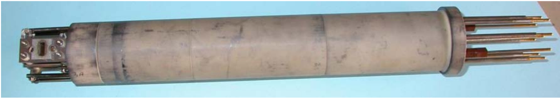
Figure 2.9. Photograph of the entire RFA probe. The electrodes are followed by \sim 18 cm long alumina body which consists of four individual cylinders. The total weight of the probe shown here is \sim 650 g, in addition to \sim 190 g of the CFC protective housing (not shown).
